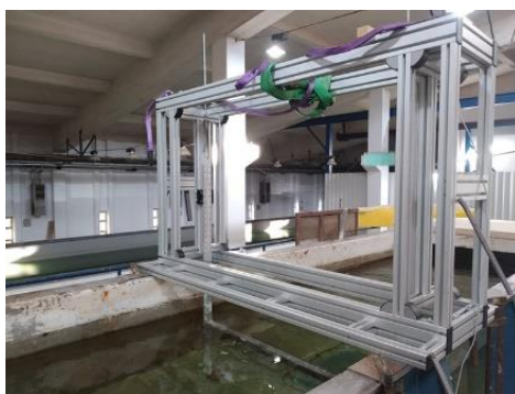
Fig. 2. The VIV test rig used in the tests.
