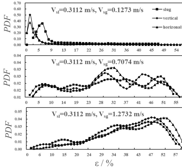
**Fig. 14. Probability density function of the gas fraction.**
