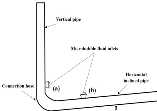
**Fig. 12. Schematic diagram of microbubble inlets.**
