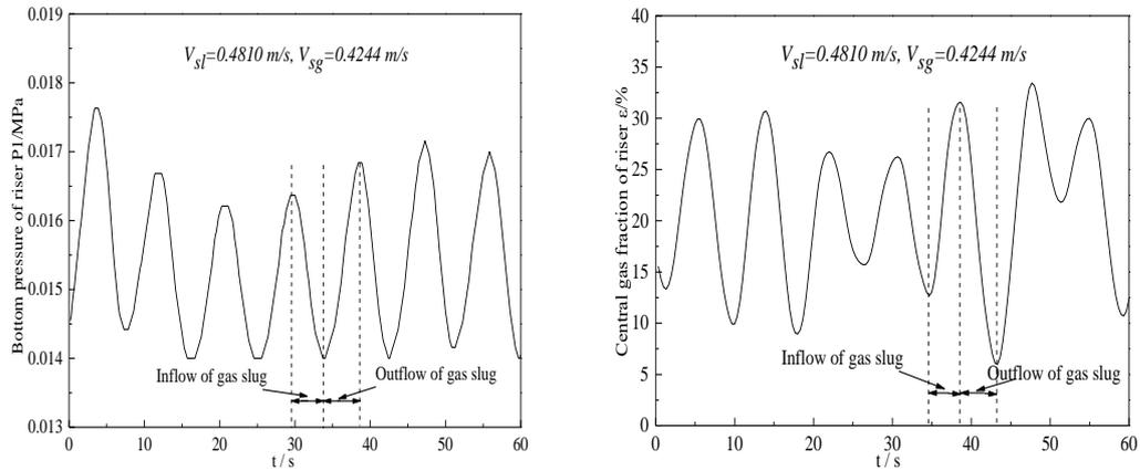
(a) Pressure fluctuations for bullet-like slug flow pattern (b) Gas fraction fluctuations for bullet-like slug flow pattern
