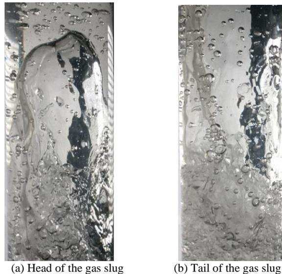
**Fig. 7. Images of the gas slug by high-speed camera for  $V_{sl}=0.4810$  m/s and  $V_{sg}=0.4244$  m/s.**
