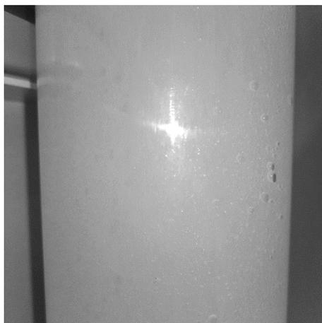
**Fig. 9.** Microbubble image in a vertical pipe.
