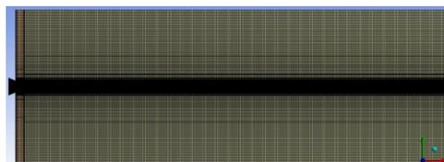
Fig. 5. Hexahedral structured mesh of the computational domain cut plane.
