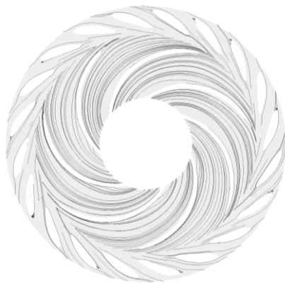
Fig. 12. Flow inside the impeller Q/Q_{opt} = 0,96 – outside hump zone.
