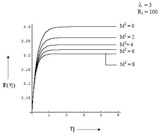
**Fig. 1.** Non-dimensional Transverse Velocity profiles for various  $M^2$
