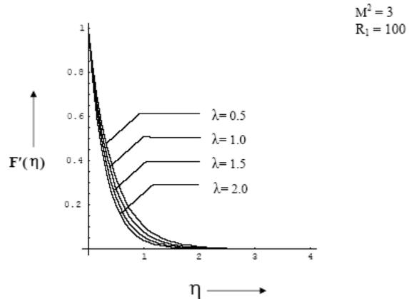
**Fig. 4.** Non-dimensional Longitudinal Velocity profiles for different  $\lambda$
