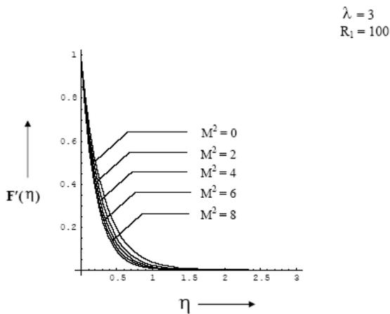
**Fig. 3.** Dimensionless longitudinal velocity profiles for various  $M^2$
