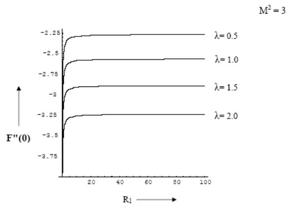
**Fig. 10.** Skin friction coefficient for various  $\lambda$
