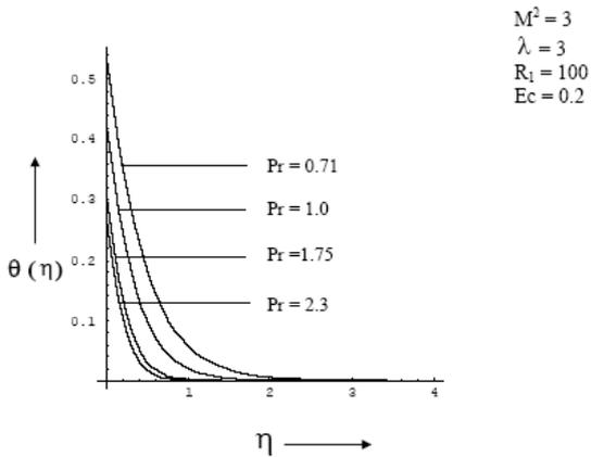
**Fig. 7.** Effect of Pr over Temperature distribution
