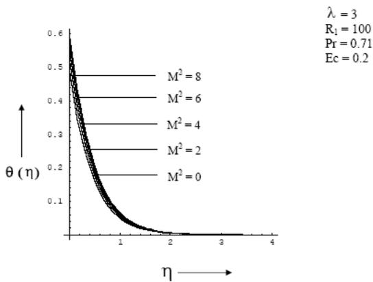
**Fig. 5.** Temperature Distribution for various values of  $M^2$
