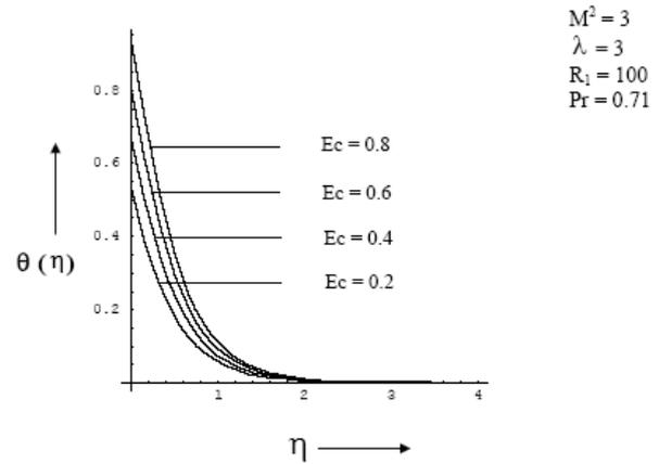
**Fig. 8.** Temperature profiles for Different Ec
