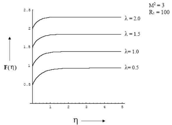
**Fig. 2.** Effect of  $\lambda$  on dimensionless Transverse Velocity
