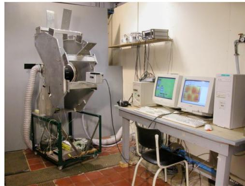
Fig. 9. Test bench for the thermal anti-icing experiments.
