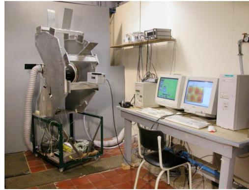
Fig. 9. Test bench for the thermal anti-icing experiments.
