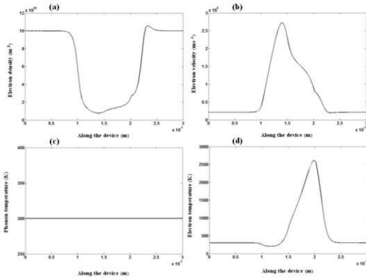
Fig. 4. Shows the distributions of electron density, (b) electron velocity, (c) lattice temperature and (d) electron temperature for voltage bias 1 V and the lattice temperature 300 K.
