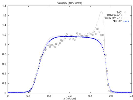
**Fig. 1.** Velocity profile ( $\times 10^7$  cm/sec) of HDM with BBW model with  $c = -1.0$  (dashed line),  $c = -2.1$  (dotted line) and with Monte-Carlo simulation (squares). The channel length is  $0.4 \mu\text{m}$ , and the applied voltage is 1V.
