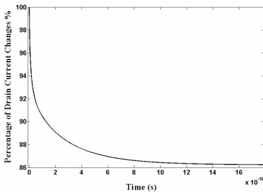
**Fig. 7.** Shows the variation of Percentage of Drain Current Changes at various times.
