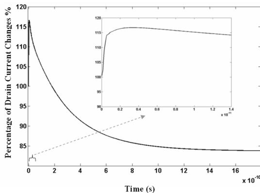
**Fig. 9.** Shows the variation of Percentage of Drain Current Changes at various times.
