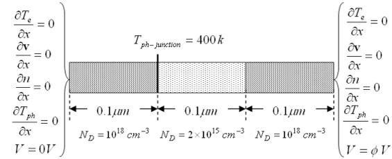
**Fig. 2.** The microscale simulation regions of a ballistic diode.
