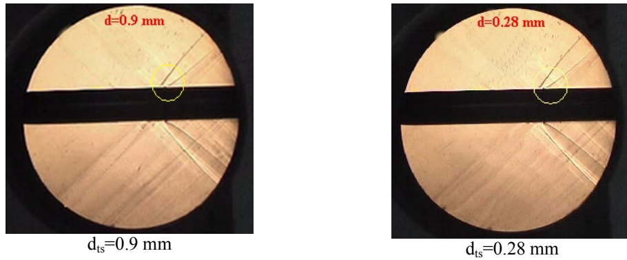
Fig. 6. Flow around cylindrical part of the Model 1 with trip strip installed at x/d=6.25 and \alpha = 0 .
