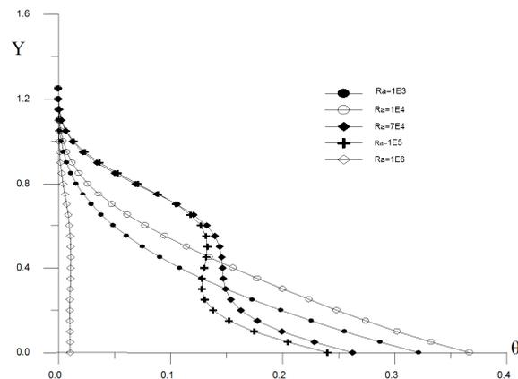
Fig. 9. Temperature profile at the middle for  $A_w=0.25$ ,  $Ra=10^3$ ;  $10^4$ ;  $7.10^4$ ;  $10^5$ ;  $10^6$
