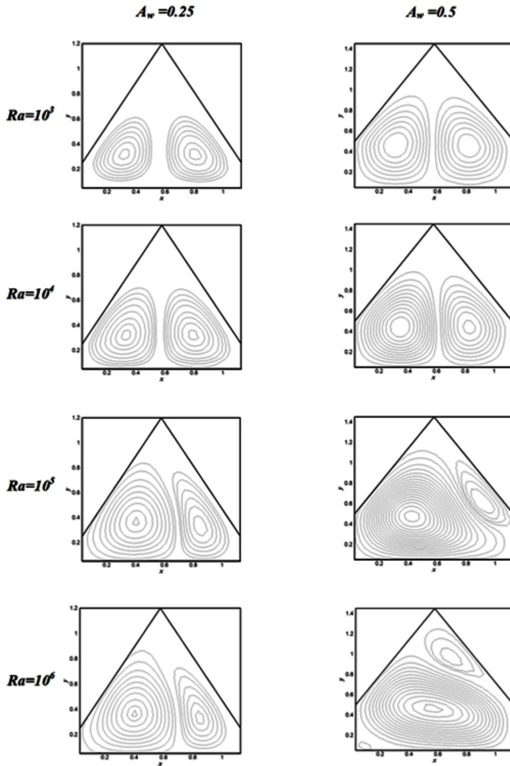
Fig. 12. Streamlines for different aspect ratios and different Rayleigh number values
