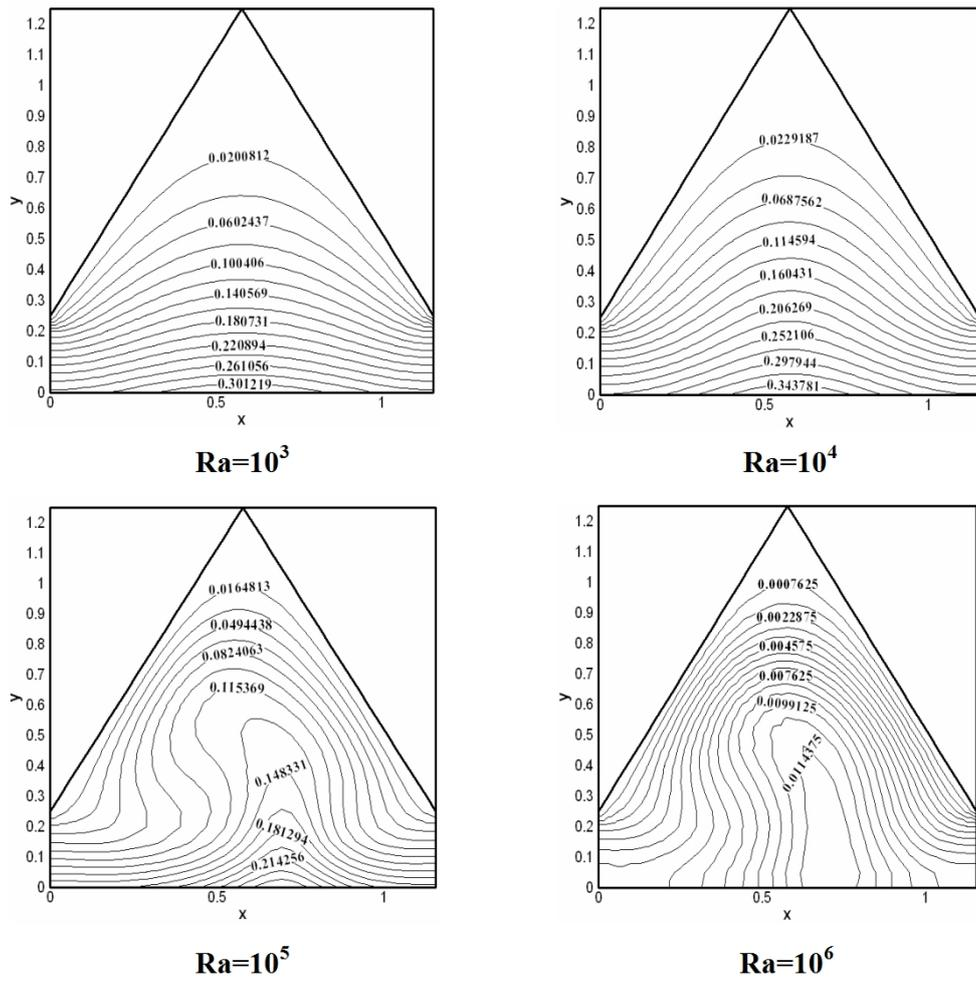
**Fig. 10.** Thermal field for  $A_w=0.25$  and different Rayleigh number values
