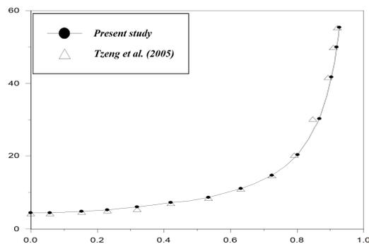
**Fig. 4.** Comparison of results of local Nusselt number for right-angle triangular enclosure
