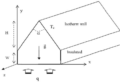
**Fig. 1.** Schematic of an air-filled prismatic cavity
