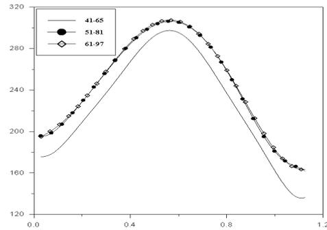
**Fig. 2.** Local Nusselt profile over the bottom surface for different numbers of meshes at  $Ra=10^6$
