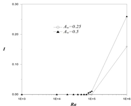
Fig. 14. Strength of asymmetry versus  $Ra$  for different aspect ratios
