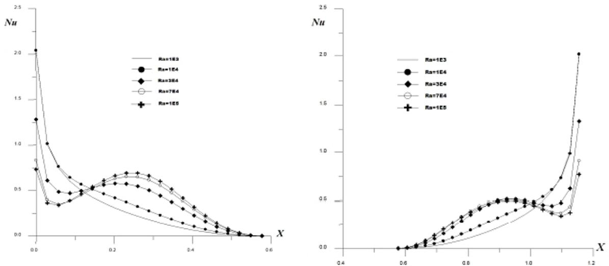
**Fig. 11.** Local Nusselt number versus X for different Rayleigh number values: left inclined wall (left) and right inclined wall (right)
