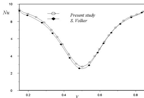
**Fig. 3.** Comparison of results of local Nusselt number on the bottom wall of a triangular cavity
