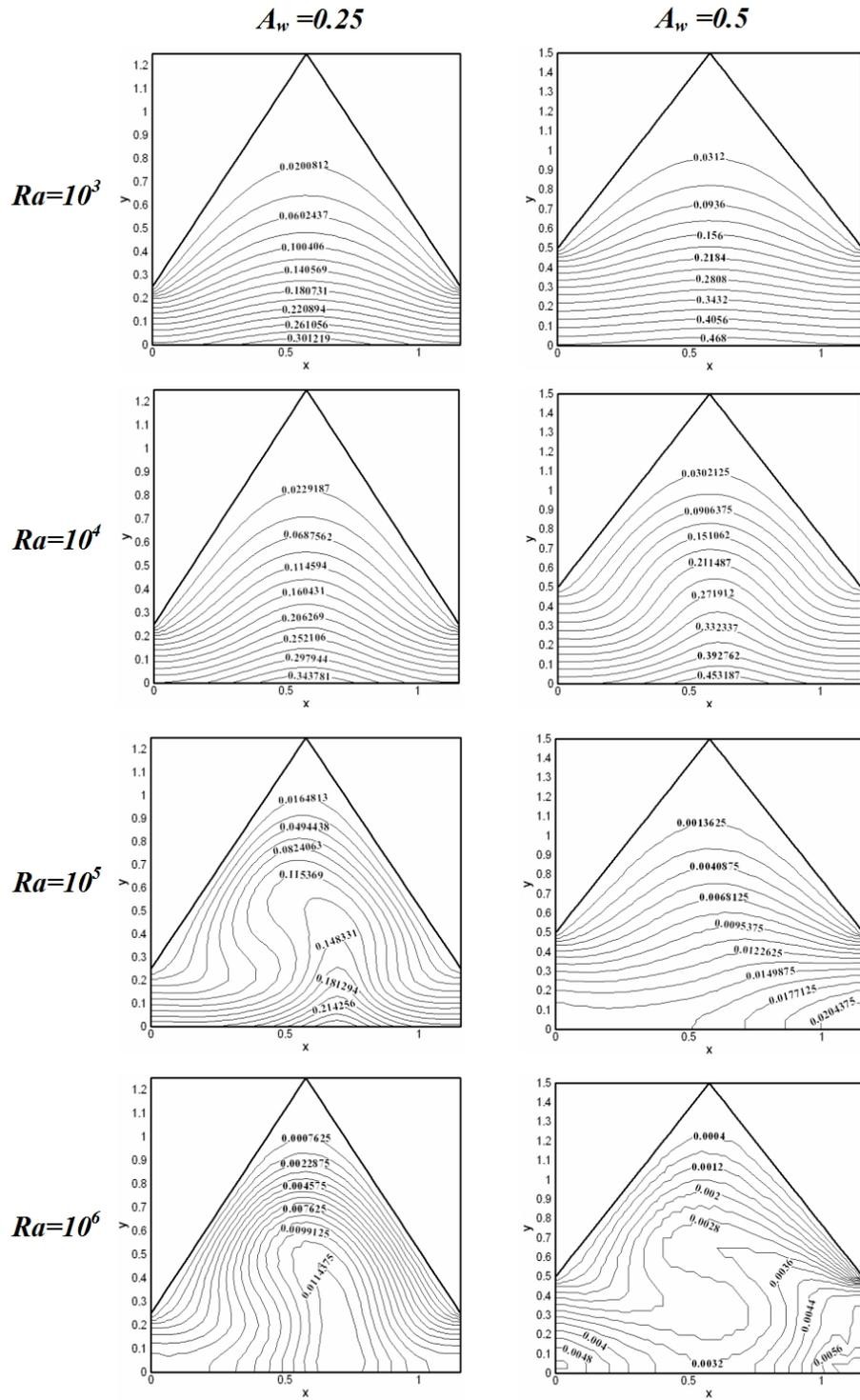
Fig. 13. Isotherms patterns for different aspect ratios and different Rayleigh number values
