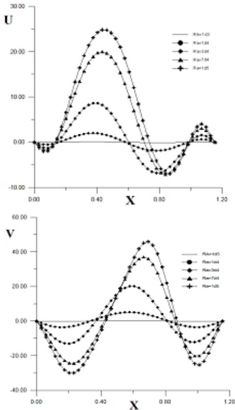
Fig. 7. Velocity components profiles along the bottom of the triangular part: horizontal component (up); vertical component (down).
