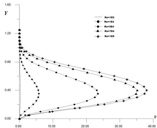
**Fig. 6.** Vertical velocity component profile at  $X=0.57$  (the middle) for  $A_w=0.25$ ;  $Ra=10^3; 10^4; 3.10^4; 7.10^4; 10^5$
