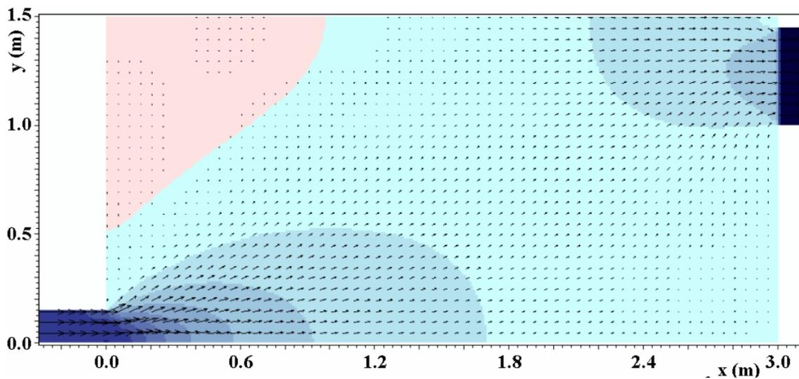
Fig.7. Instantaneous simulated field at 16 min 40 s, with constant turbulent viscosity of  $0.01 \text{ m}^2/\text{s}$ . The colors follow the same scale of Fig. 3, and corresponds to the “x component” of the velocity.
