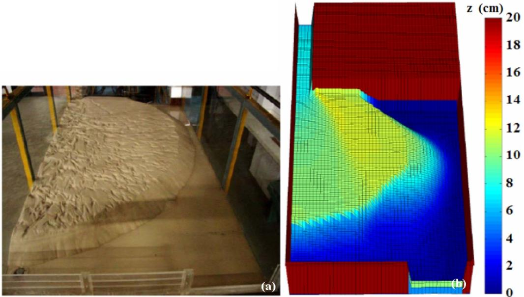
Fig.12. Observed (a) and predicted (b) sand bed after 72 h. The color scale indicates  $z$  (cm), the height of the bed. The experiment (a) shows microchannels (lower bed level) concentrated closer to the left wall, which coincides with the position of the lower level of the simulated sand bed (b).
