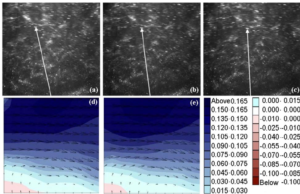
**Fig.3.** A sequence of flow images is shown in (a), (b) and (c). The arrows show the same particle in the sequence. (d) and (e) are instantaneous flow fields obtained with the previous pictures. Color scale is for the x velocity component in (m/s) (horizontal axis in this figure).
