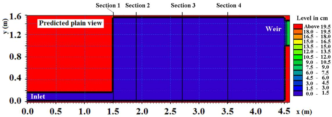
Fig.8. Sand reservoir before the sediment transport simulation. The color scale is also valid for Figs. 9, 10 and 11.
