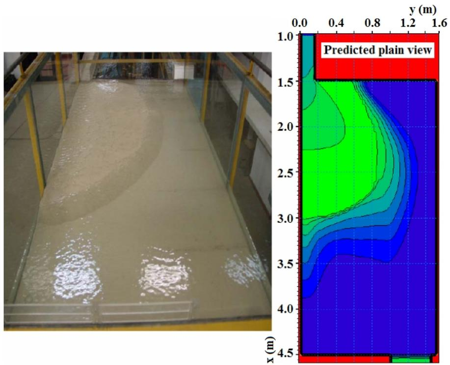
Fig.11. Observed and predicted sand bed after 50h.
