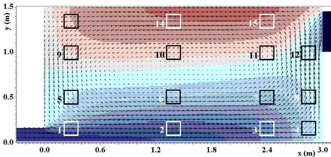
Fig.5. Predicted mean flow pattern, with PIV measurement regions identified by numbered squares. The colors correspond to the “x component” of the velocity. Color scale in Fig.3.
