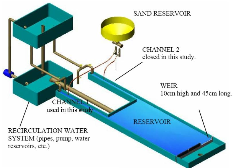
**Fig.1.** Above: view of the reservoir. Below: simplified sketch of the reservoir.
