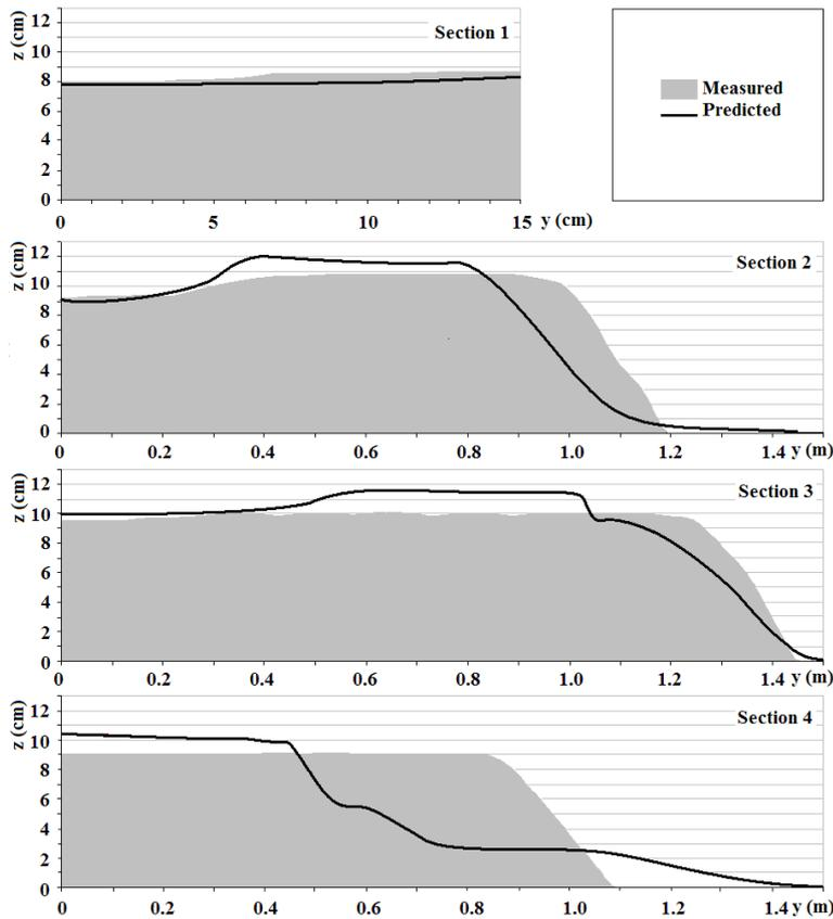
Figure 13 – Comparison of predicted and measured bed profiles in sections 1 through 4 after 72h.
