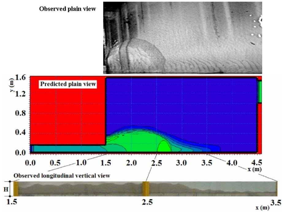
Fig.10. Predicted and observed sand bed after 20h. H is the position of the water surface.
