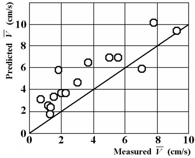
Fig.6. Predicted and measured velocities.  $\bar{V}$  is the module of the mean velocity vector.
