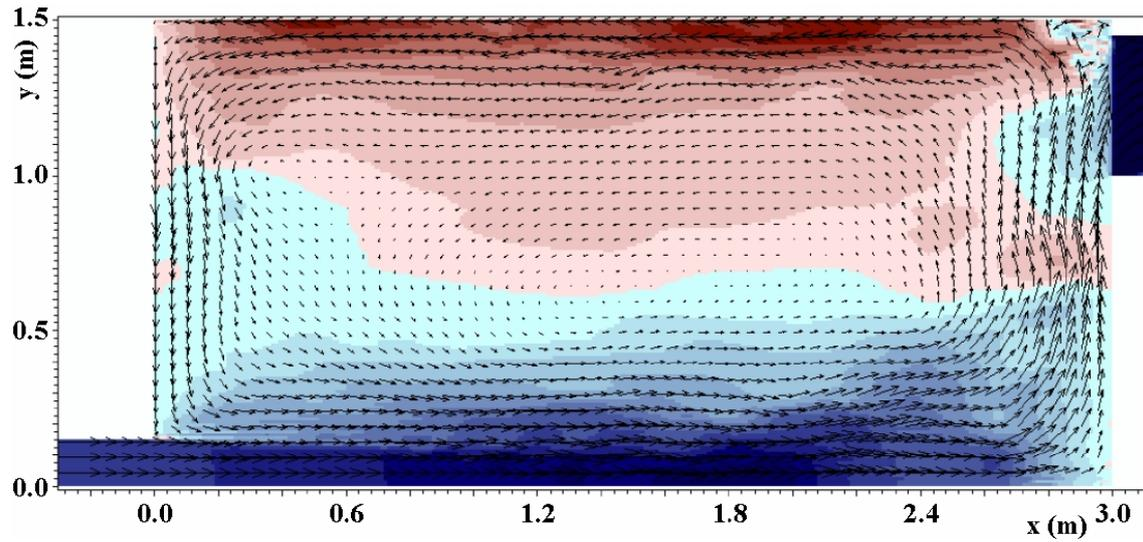
Fig.4. Instantaneous simulated field at 16 min 40 s. The colors follow the same scale of Fig. 3, and corresponds to the “x component” of the velocity.
