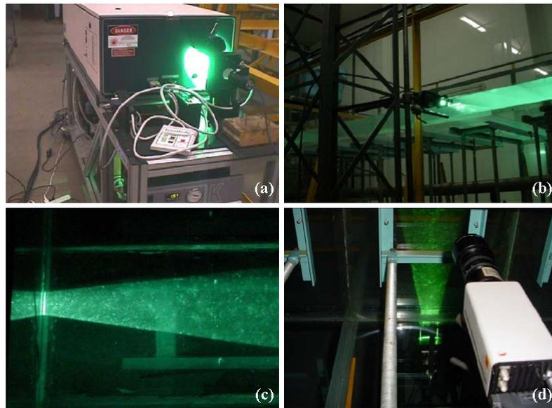
**Fig.2.** Laser equipment in operation. (a) The 20W laser source. (b) Laser sheet applied through a lateral wall of the reservoir. (c) Plain view of the laser sheet in the reservoir. (d) CCD camera positioned beneath the reservoir bed. The camera was connected to a computer, for the analysis of images and calculus of instantaneous and mean velocity fields.
