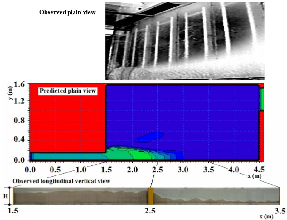
Fig.9. Predicted and observed sand bed after 10h. H is the position of the water surface, which varied from 11,5cm to 12,5cm above the horizontal bed.
