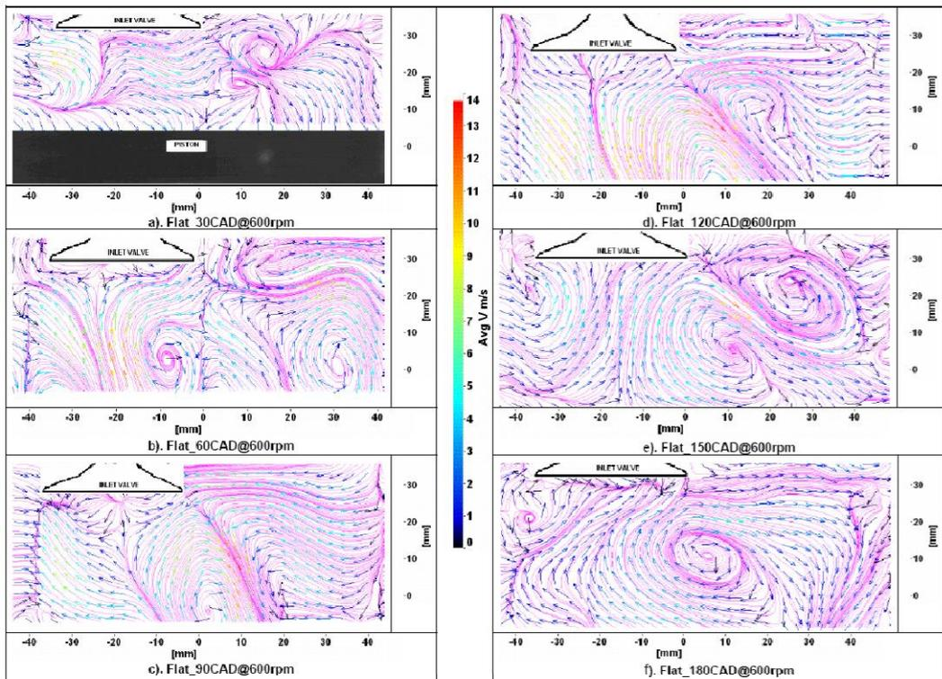
**Fig. 5.** The ensemble average velocity vectors during intake stroke at an engine speed of 600 rev/min.
