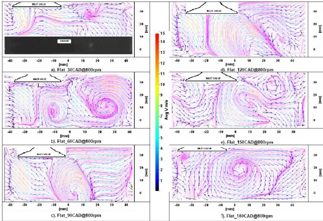
**Fig. 6.** The ensemble average velocity vectors during intake at an engine speed of 800 rev/min.
