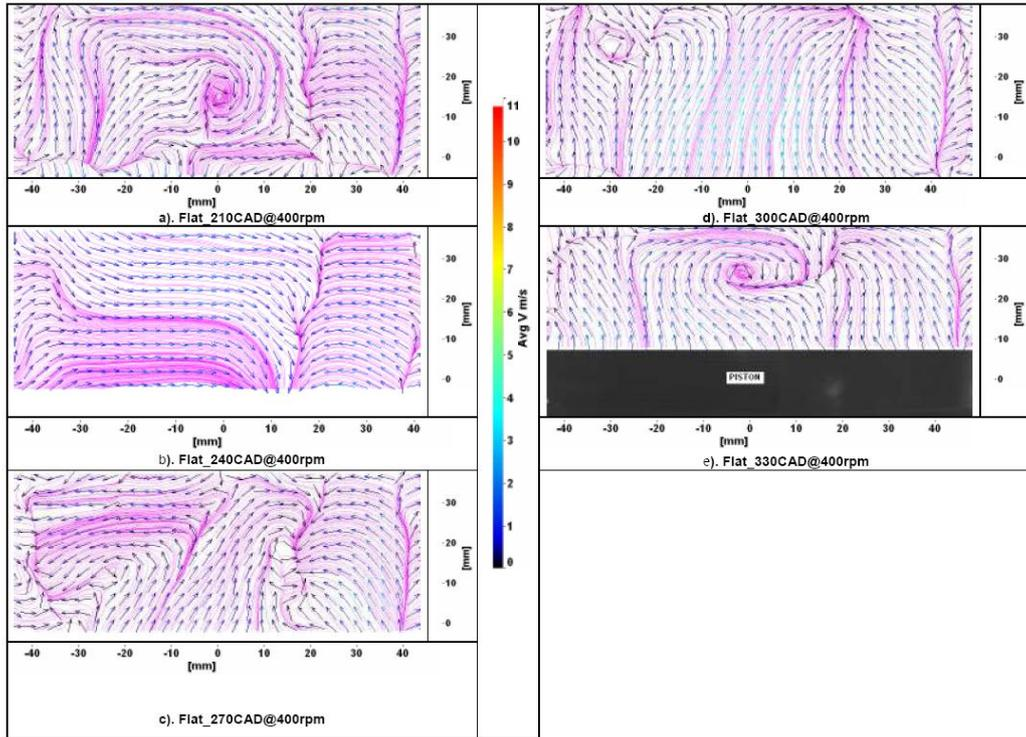
**Fig. 8.** The ensemble average velocity vectors during compression stroke at an engine speed of 400 rev/min.
