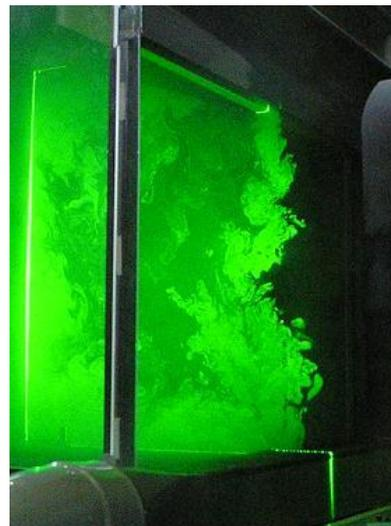
**Fig. 4.** Flow visualization by laser tomography (seeding in the jet)
