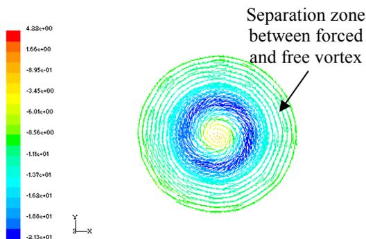
Fig. 6b. Projected velocity vectors at  $z = 765\text{ mm}$ , (units of colored scale in m/s).
