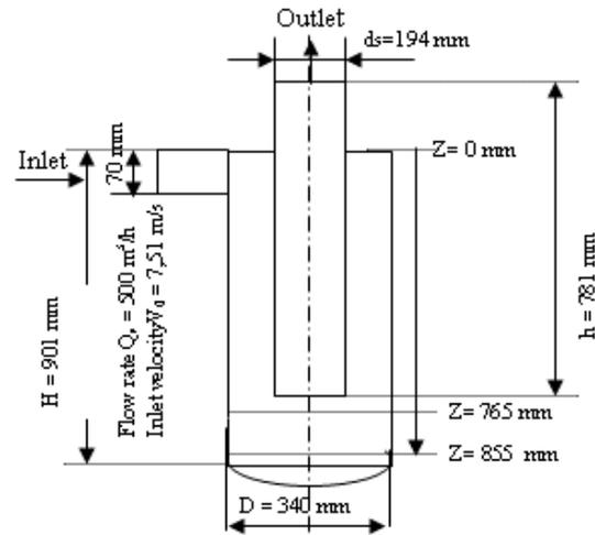
Fig. 2. Axial measuring positions under the vortex finder.
