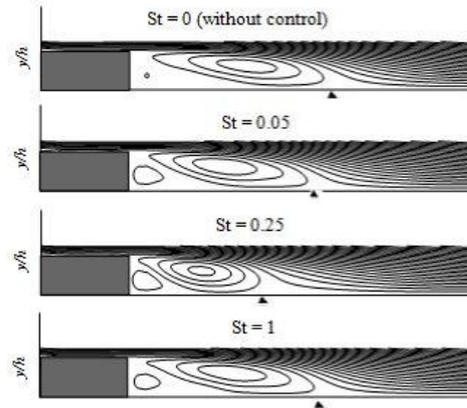
**Fig.4.** Iso-stream function lines for different Strouhal number  $St$ .
