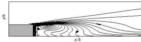
**Fig. 3.** Distributions of iso-concentration lines.  $Re = 33000$ , without control
