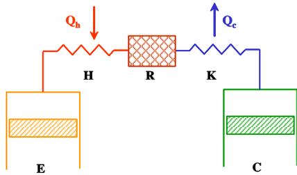
Fig. 2. Principle of the Stirling engine
