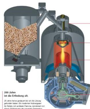
**Fig. 17.** The wood pellets Sunmachine micro-cogenerator (Source: [www.sunmachine.de](http://www.sunmachine.de))
