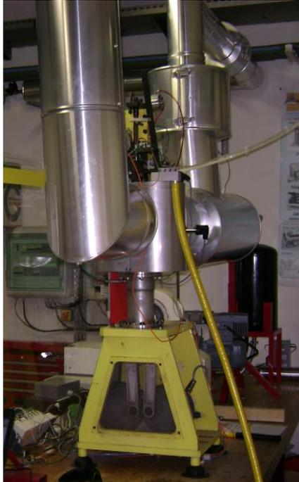
**Fig. 20.** The prototype of the 'hot' part of the Ericsson engine
