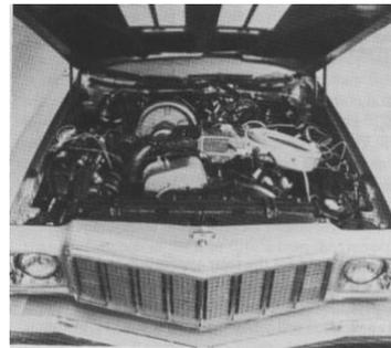
**Fig. 12.** Ford's 4-215 Stirling engine in a Ford Taunus
