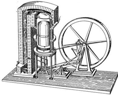
**Fig. 6.** The first Stirling engine (1816)
