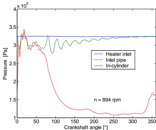
**Fig. 21.** Pressure evolution for an inlet temperature of  $518^\circ\text{C}$
