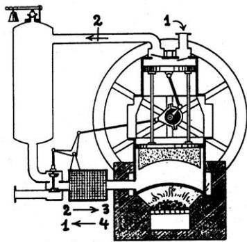
**Fig. 8.** The open cycle Ericsson engine (1853) (Kolin, 1991)
