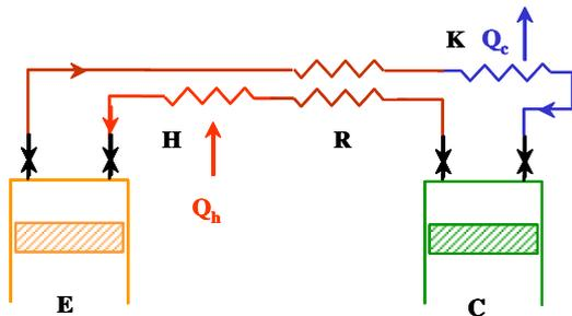
Fig. 3. Principle of the Ericsson engine
