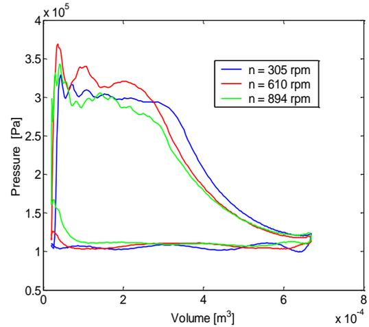
**Fig. 22.** Indicated diagrams for an inlet temperature of  $518^\circ\text{C}$  and for three rotational speeds.
