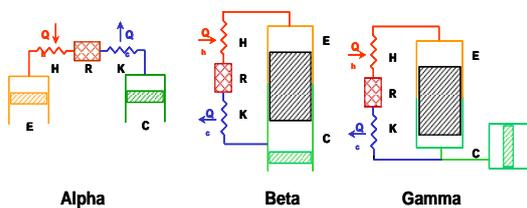
Fig. 4. Stirling engine basic geometrical configurations
