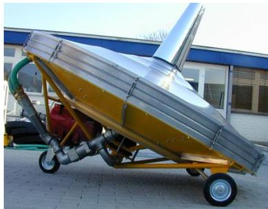
Fig. 19. A low  $\Delta T$  solar engine (Source: [www.bsrsolar.com](http://www.bsrsolar.com))
