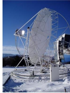
**Fig. 14.** Solar Dish/Stirling technology system (Source: CNRS-PROMES, Font-Romeu, France)
