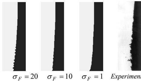
**Fig. 6.** Numerical and experimental results for plane jet spreading
