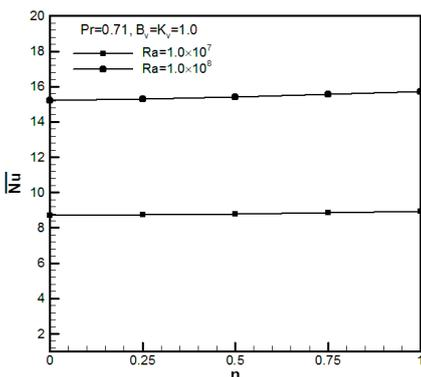
**Fig. 8.** The effect of microrotation boundary condition on the average Nusselt number,  $\overline{Nu}$ , for  $K_v = 1.0$ ,  $B_v = 1.0$  and  $Pr=0.71$ .
