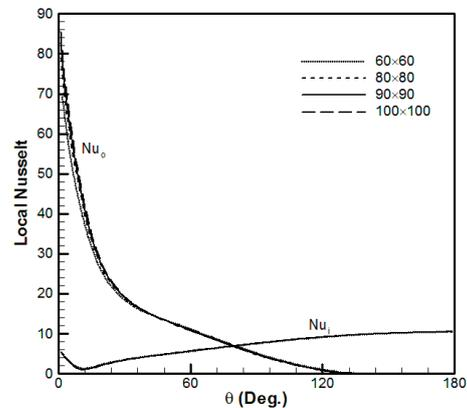
Fig. 2. Variation of local Nusselt number over the cold boundary for various mesh sizes and for  $Ra=5 \times 10^7$ ,  $Pr=0.71$ ,  $K_v=0.1$ ,  $B_v=1.0$  and  $R^*=2.0$ .
