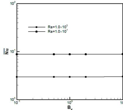
**Fig. 9.** The effect of dimensionless microinertia  $B_v$  on the average Nusselt number,  $\overline{Nu}$ , for  $K_v = 1.0$  and  $Pr=0.71$ .
