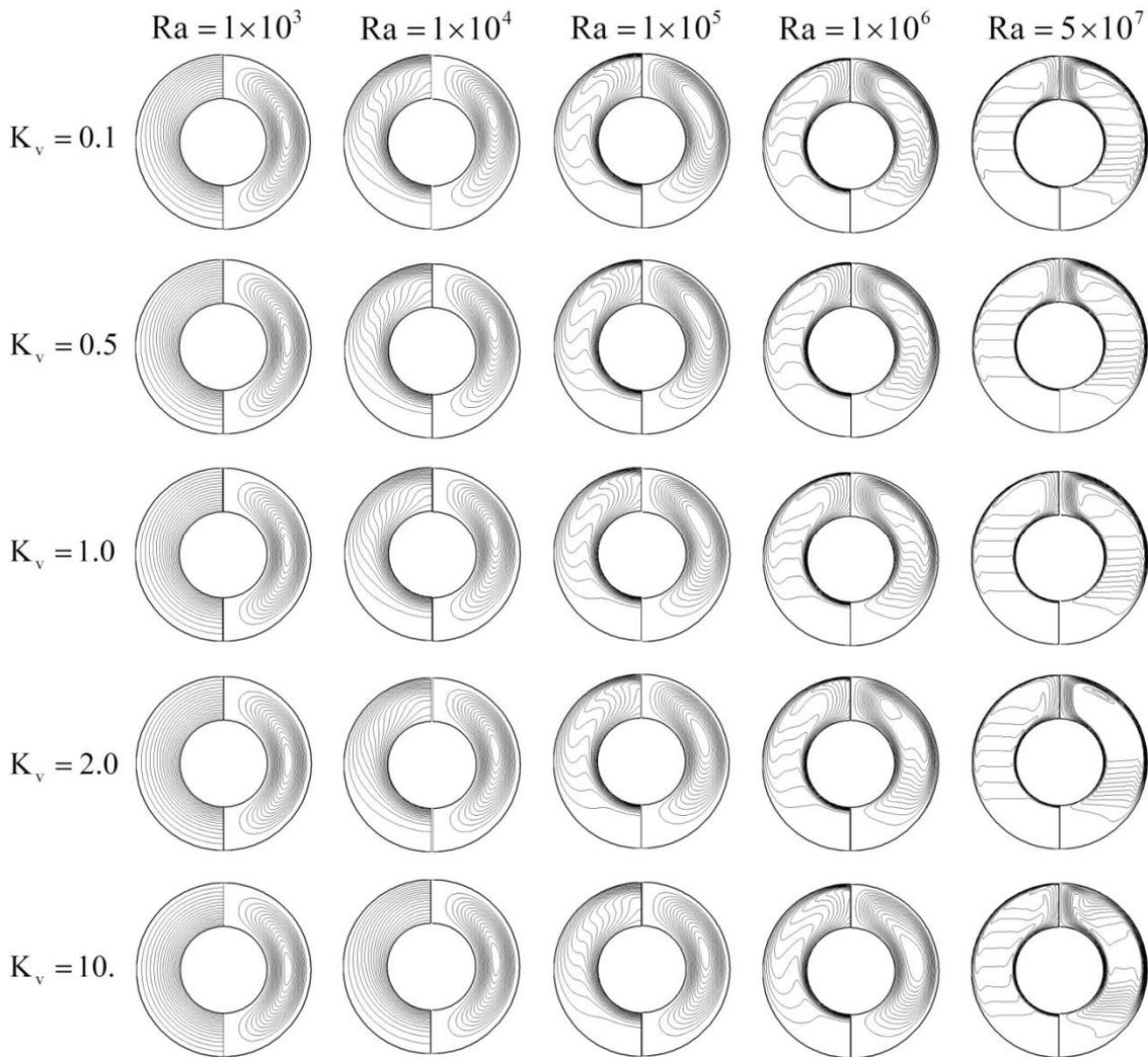
**Fig. 4.** Isotherms and streamlines for different material parameters  $K_v$  and different Rayleigh number values ( $Pr=0.71$ ,  $B_v=1.0$  and  $n=0.5$ )
