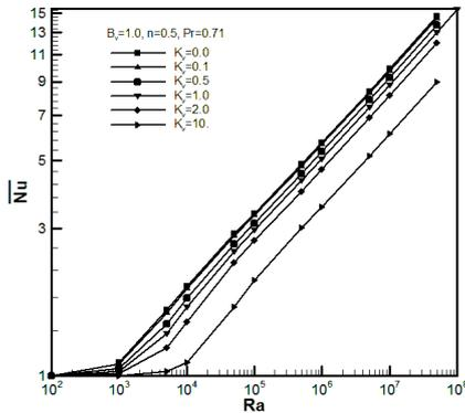
**Fig. 6.** Variation of average Nusselt number  $\overline{Nu}$  with Rayleigh number for different material parameters  $K_v$ ,  $Pr=0.71$ ,  $B_v = 1.0$  and  $n = 1/2$ .
