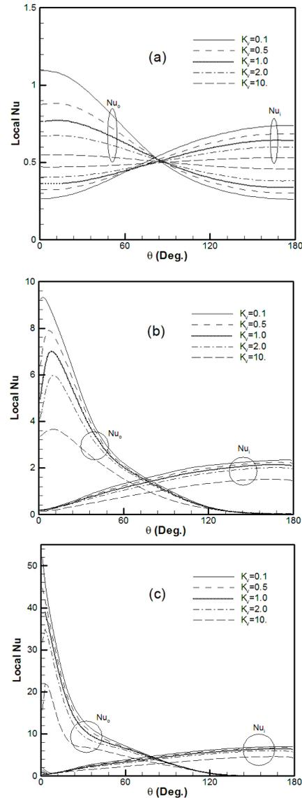
Fig. 5. Distribution of the local Nusselt number for various values of vortex viscosity ratio,  $K_v$ , at inner and outer spheres and for Rayleigh number (a)  $10^3$ , (b)  $10^5$  and (c)  $10^7$ .
