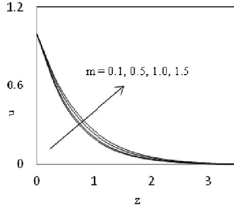
Fig. 4. The primary velocity 'u' versus 'z' for  $M = 1.0$ ,  $\Omega = 0.4$ ,  $t = 1$
