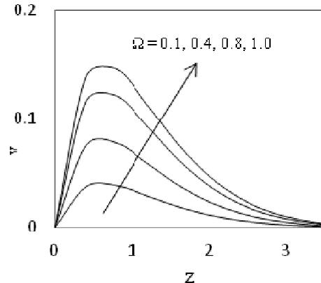
Fig. 5. The secondary velocity 'v' versus 'z' for  $M = 1.0$ ,  $m = 0.5$ ,  $t = 1$
