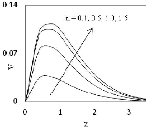
Fig. 7. The secondary velocity 'v' versus 'z' for  $M = 1.0, \Omega = 0.4, t = 1$
