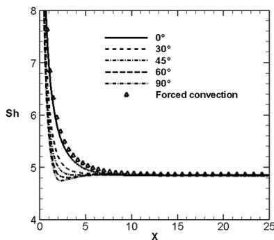
Fig. 12. Axial evolution of Sherwood number at the lower wet plate
