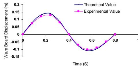
**Fig. 5.** Experimental and theoretical wave board displacement for generating a wave of about 1-m length
