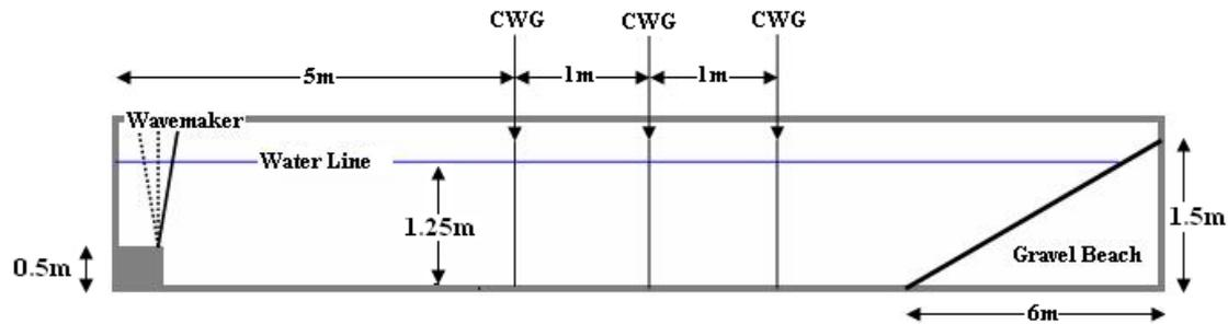
Fig. 2. The configuration of wave gauges and other equipments in the wave flume.
