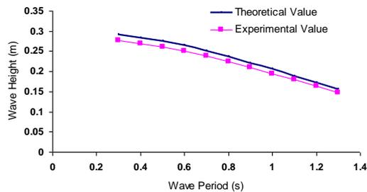
**Fig. 4.** Experimental and theoretical wave-maker characteristic for regular waves.
