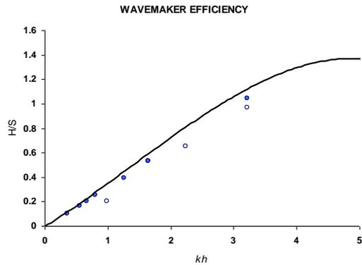
**Fig. 3.** Experimental wave height ( $H$ ) to stroke ( $S$ ) ratio plotted against relative depth ( $kh$ ). The solid line represents the theoretical ratio, while the open and solid circles are experimental data before and after sealing leaks around paddle respectively
