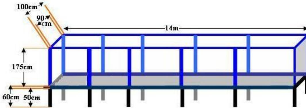
Fig. 1. 3D view of wave flume design
