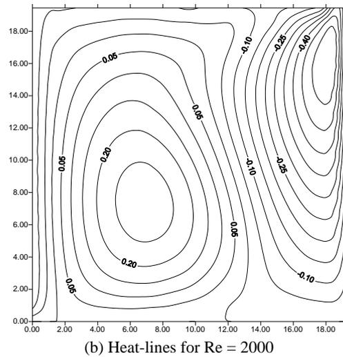
**Fig. 7.** Heat-lines for Case II at buoyancy ratio = 0.1
