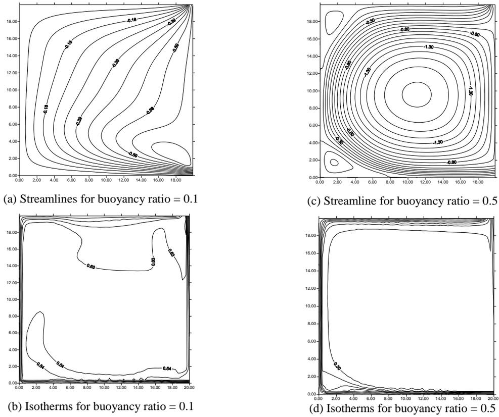
**Fig. 3.** Streamlines and isotherms for Case I at  $Re = 2000$
