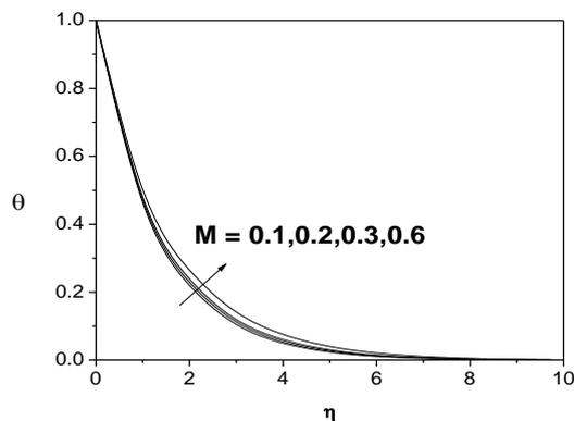
**Fig. 7.** Variation of the velocity component  $\theta$  with  $M$  for  $Pr=0.72$ ,  $Sc=0.62$ ,  $Gt=Gc=Fw=K=0.1$ .
