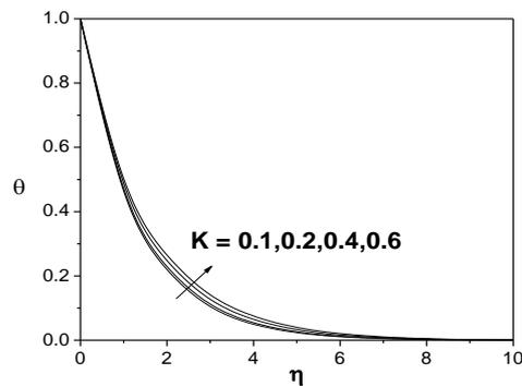
**Fig. 12.** Variation of the temperature  $\theta$  with  $K$  for  $Pr=0.72, Sc=0.62, Gt=Gc=Fw=M=0.1$ .
