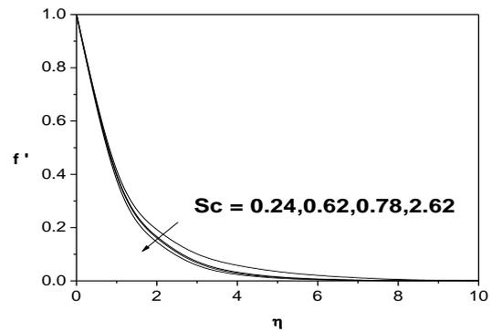
**Fig. 5.** Variation of the velocity component  $f'$  with  $Sc$  for  $Pr=0.72, Gt=Gc=Fw=M=K=0.1$ .
