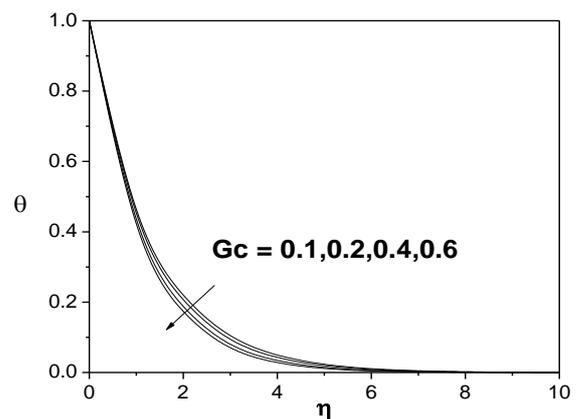
**Fig. 9.** Variation of the temperature  $\theta$  with  $Gc$  for  $Pr=0.72$ ,  $Sc=0.62$ ,  $Gt=Fw=M=K=0.1$ .
