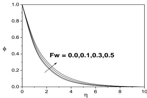
**Fig. 16.** Variation of the concentration  $\phi$  with  $F_w$  for  $Pr=0.72, Sc=0.62, Gt=Gc=M=K=0.1$ .
