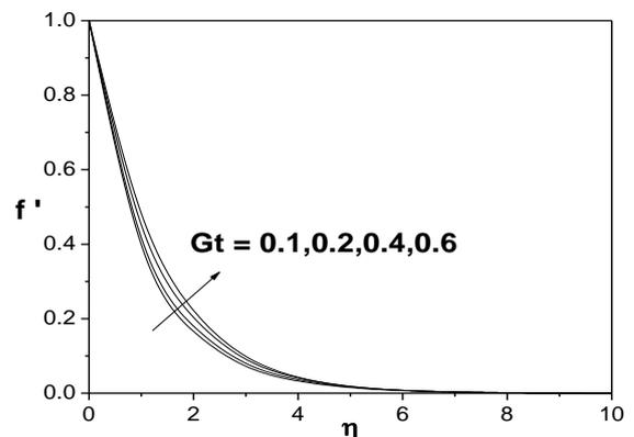
**Fig. 2.** Variation of the velocity component  $f'$  with  $Gt$  For  $Pr=0.72$ ,  $Sc=0.62$ ,  $Gc=M=Fw=K=0.1$ .
