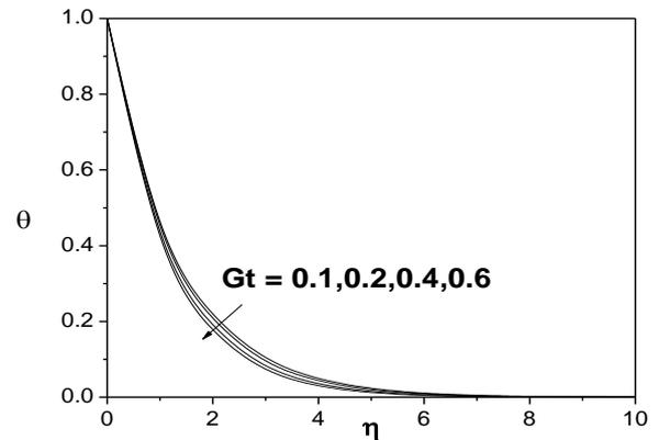
**Fig. 8.** Variation of the temperature  $\theta$  with  $Gt$  for  $Pr=0.72$ ,  $Sc=0.62$ ,  $Fw=Gc=M=K=0.1$ .
