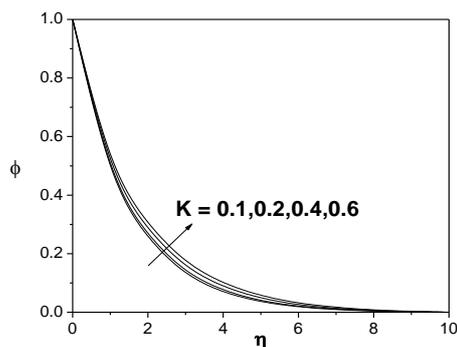
**Fig. 18.** Variation of the concentration  $\phi$  with  $K$  for  $Pr=0.72, Sc=0.62, Gt=Gc=Fw=M=0.1$ .
