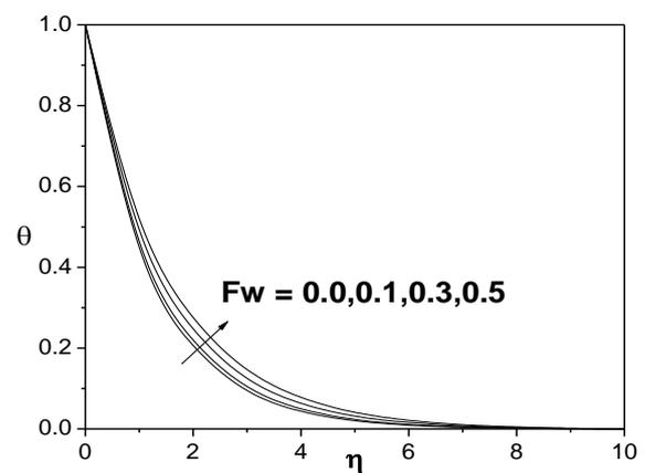
**Fig. 10.** Variation of the temperature  $\theta$  with  $Fw$  for  $Pr=0.72$ ,  $Sc=0.62$ ,  $Gc=Gt=M=K=0.1$ .
