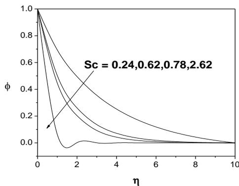
**Fig. 17.** Variation of the concentration  $\phi$  with  $Sc$  for  $Pr=0.72, Gt=Gc=Fw=M=K=0.1$ .
