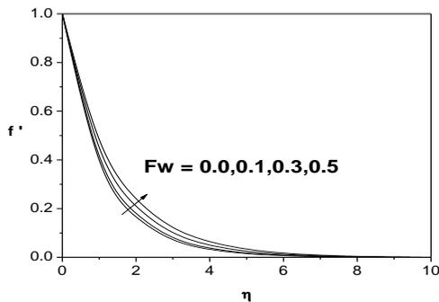
**Fig. 4.** Variation of the velocity component  $f'$  with  $Fw$  for  $Pr=0.72, Sc=0.62, Gc=Gt=M=K=0.1$ .
