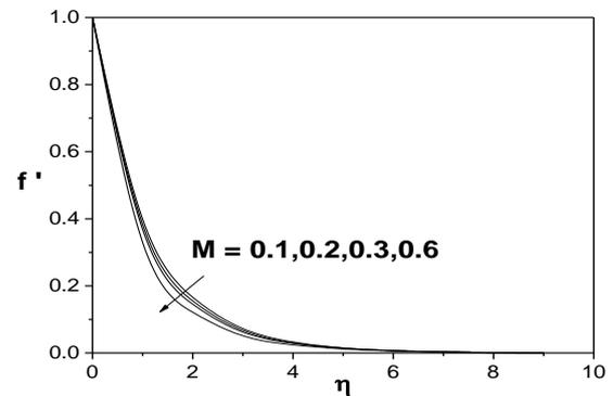
**Fig. 1.** Variation of the velocity component  $f'$  with  $M$  for  $Pr=0.72$ ,  $Sc=0.62$ ,  $Gt=Gc=Fw=0.1$ ,  $K=0.1$ .
