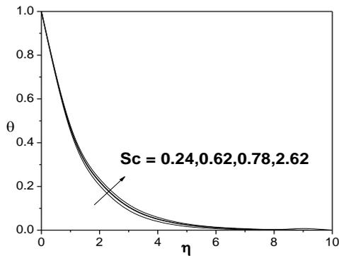
**Fig. 11.** Variation of the temperature  $\theta$  with  $Sc$  for  $Pr=0.72, Gt=Gc=Fw=M=K=0.1$ .
