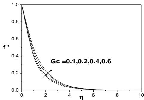
**Fig. 3.** Variation of the velocity component  $f'$  with  $Gc$  for  $Pr=0.72, Sc=0.62, Gt=Fw=M=K=0.1$ .
