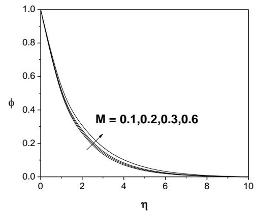
**Fig. 13.** Variation of the concentration  $\phi$  with  $M$  for  $Pr=0.72, Sc=0.62, Gt=Gc=Fw=K=0.1$
