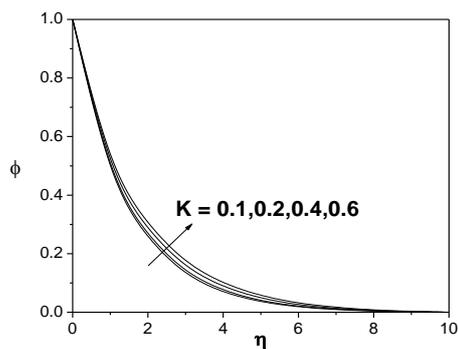
**Fig. 18.** Variation of the concentration  $\phi$  with  $K$  for  $Pr=0.72, Sc=0.62, Gt=Gc=Fw=M=0.1$ .
