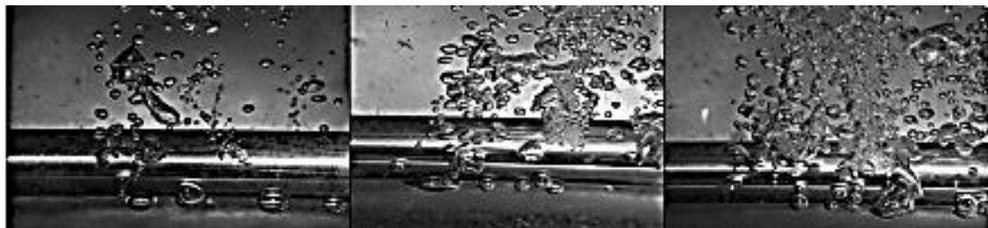
a) Heat flux  $15 \text{ kw/m}^2$     (b) Heat Flux  $40 \text{ kw/m}^2$     (c) Heat flux  $90 \text{ kw/m}^2$
