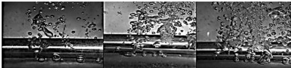
a) Heat flux 15kW/m (b) Heat Flux 40 kW/m<sup>2</sup> (c) Heat flux 90kW/m<sup>2</sup>
