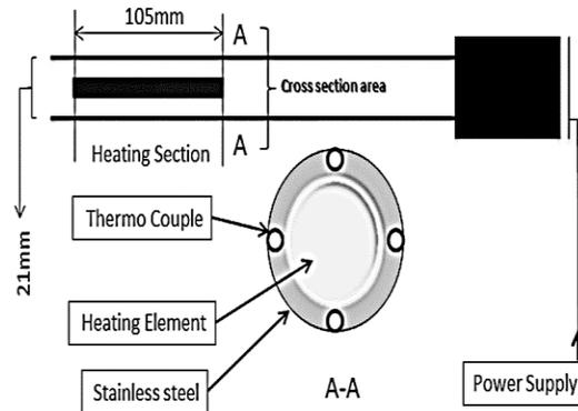
**Fig. 2.** Some details of heating section
