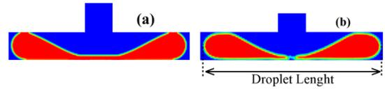
**Fig. 8.** a) Piecewise linear profile of the droplets during the breakup for the nanoscale case. b) Definition of length of droplet breakup.
