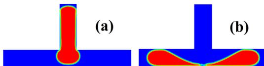
**Fig. 4.** The breakup of droplet in a T-junction. The breakup time is the time of the whole procedure between figure (a) and figure (b).
