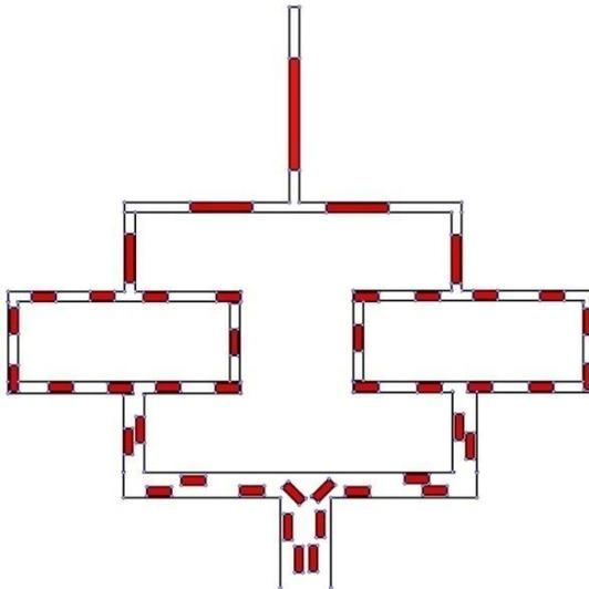
**Fig. 3.** A schematic figure of production of large number of droplets in consecutive T-junctions.
