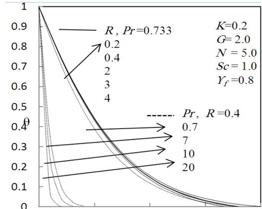
Fig. 7. Temperature profile for different values of R and different values of Pr
