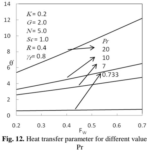
**Fig. 12.** Heat transfer parameter for different values of Pr
