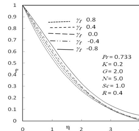
Fig. 8. Velocity profile for different variable viscosity
