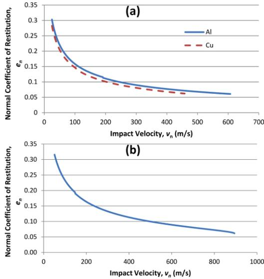
**Fig. 3.** (a) Calculated values of normal coefficient of restitution as a function of impact velocity for 30-micron aluminum and copper particles, (b) Normal coefficient of restitution as a function of impact velocity for 1.6-mm hardened steel particles.
