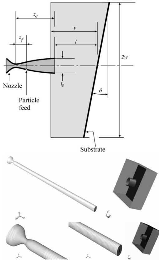
Fig. 1. Calculation domain for the simulation (not to scale.)
