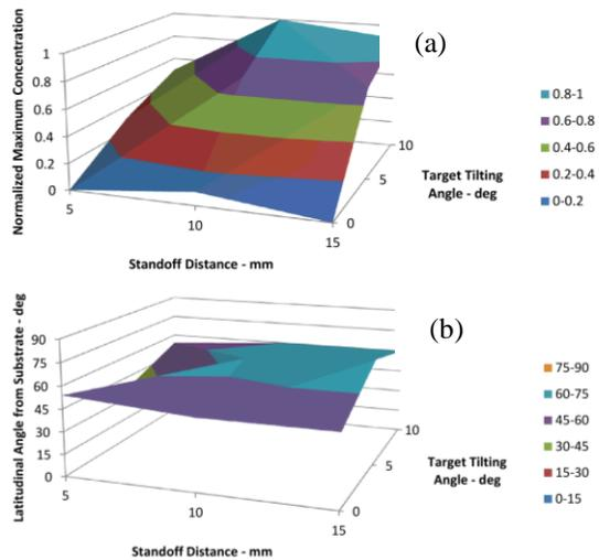
**Fig. 11.** Quantitative representation of results for aluminum particles and a spray temperature of 100 °C, representing the effect of target tilting angle and standoff distance on (a) normalized maximum particle concentration and (b) latitudinal angle of the spot from substrate, deg.
