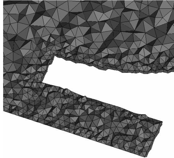
**Fig. 2.** The computational mesh near the burner region of the regeneration reactor.
