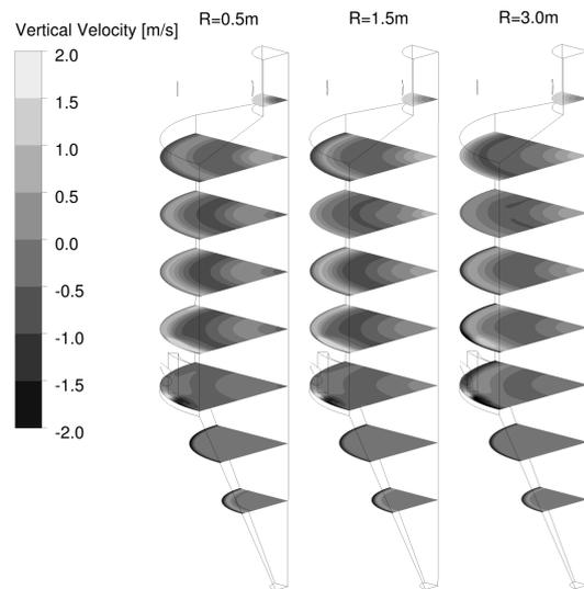
**Fig. 4.** Vertical velocity distribution in the process for the different nozzle positions, 0.5 m, 1.5 m and 3.0 m from the center.
