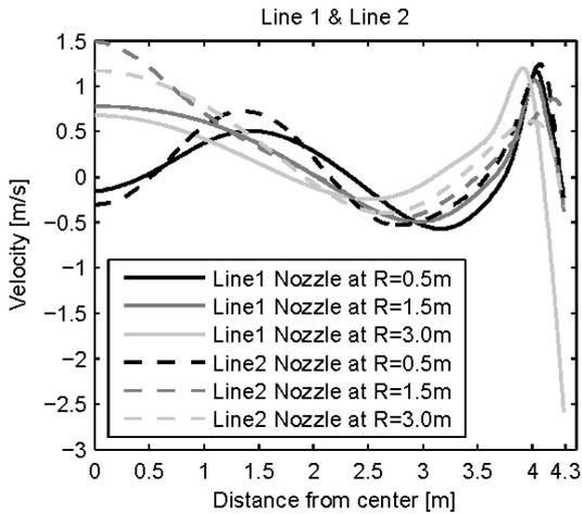
**Fig. 7.** Vertical velocities along two lines, Line 1 and Line 2, perpendicular to the wall, 8.8 m and 11.0 m from bottom.
