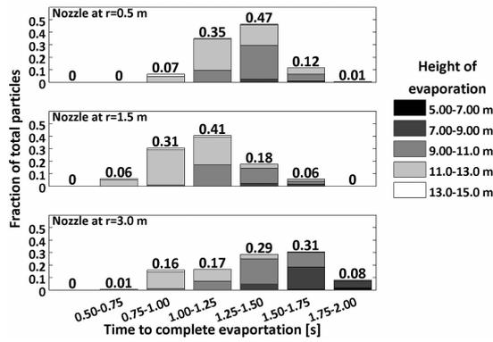
**Fig. 5.** Height position of fully evaporated particles. Each panel (diagram) represents different nozzle positions (from top to bottom):  $r = 0.5$  m,  $r = 1.5$  m and  $r = 3.0$  m respectively. The y and x axes show the fraction of particles and time until fully evaporated and the grey scale indicates at which height the particles are evaporated.
