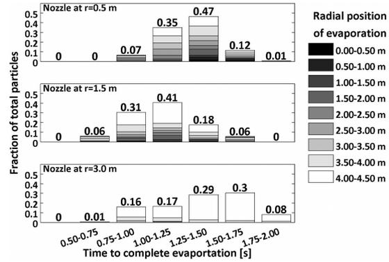
**Fig. 6.** Radial position of fully evaporated particles. Each panel (diagram) represents different nozzle positions (from top to bottom):  $r = 0.5$  m,  $r = 1.5$  m and  $r = 3.0$  m respectively. The y and x axes show the fraction of particles and time until fully evaporation, respectively, while the grey scale indicates at which radial position the particles are evaporated.
