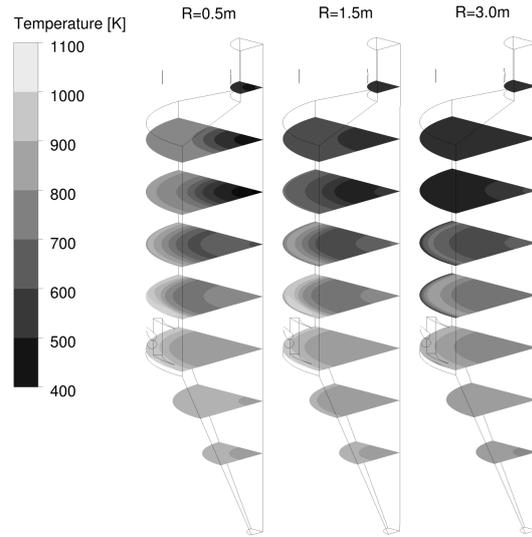
**Fig. 3.** Temperature distribution of the process for the different simulated cases with nozzle position at 0.5 m, 1.5 m and 3 m from center.
