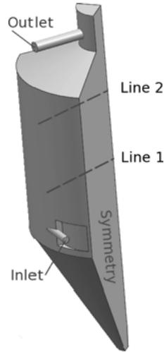
**Fig. 1.** Schematic view of the reactor geometry represented by one quarter of the domain. The spray roasting process is driven by the four burners placed along the periphery of the reactor. Waste acid is injected through spray nozzles at the top of the reactor. Chloride gas is collected at the outflow location while precipitated solid iron oxide falls to the bottom of the reactor, where it is collected.
