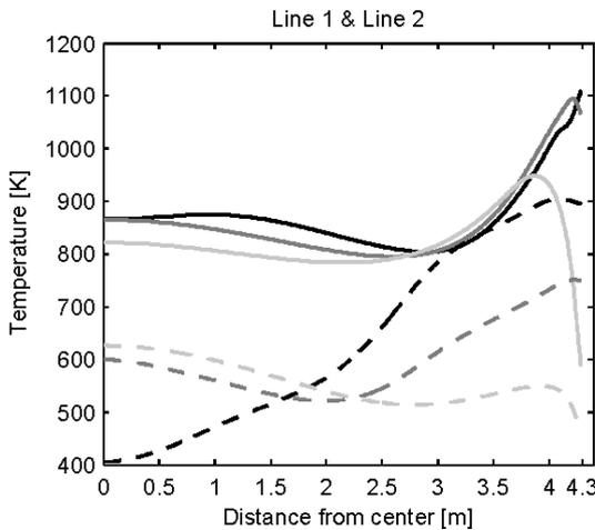
**Fig. 8.** Temperature along two lines, Line 1 and Line 2, perpendicular to the wall, 8.8 m and 11.0 m from bottom. Legends as in Fig. 7.
