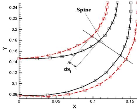
Fig. 3. Schematic of ball displacement along spine
