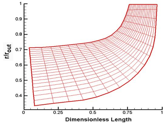
**Fig. 6.** Hub-to-shroud profile of radial impeller with its streamlines
