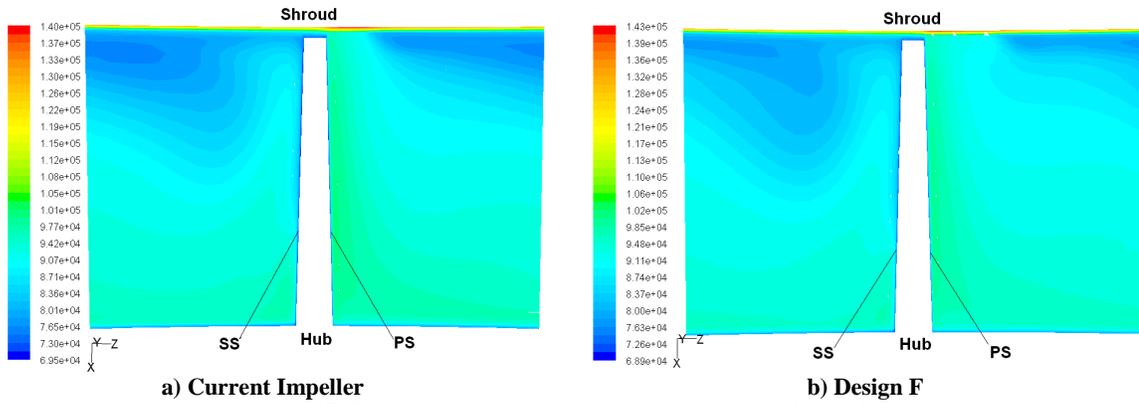
Fig. 33. Relative stagnation pressure contour on the impeller outlet
