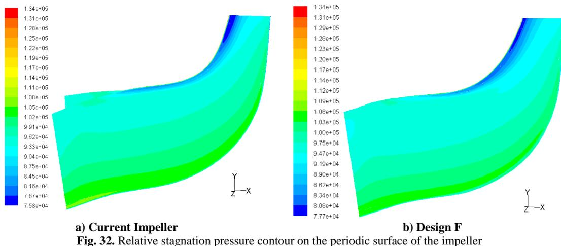
Fig. 32. Relative stagnation pressure contour on the periodic surface of the impeller
