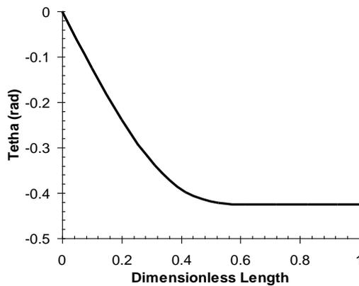
**Fig. 5.** Mean blade shape for radial impeller
