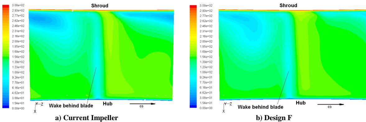
Fig. 34. Relative velocity contour on the impeller outlet
