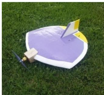
**Fig. 13. Ready to fly tests MAV**
