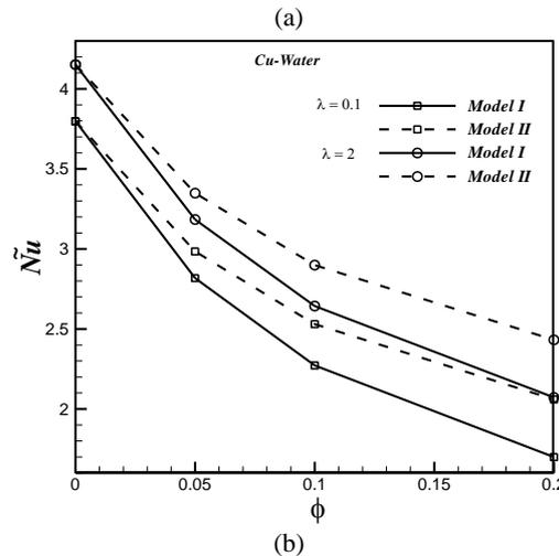
**Fig. 4.(a) Temperature distribution for different types of nanofluids when  $K_i=0.1, \phi=0.1, \varepsilon=0.1, \gamma=0.5, \lambda=0.1$  and  $Pr=6.2$ ; (b) Variation in Nusselt number with nanoparticle volume fraction for different models  $K_i=0.1, \varepsilon=0.1, \gamma=0.5$  and  $Pr=6.2$ .**
