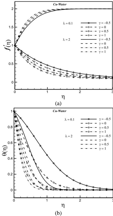
**Fig. 3. Effect of Suction or injection parameter ( $\gamma$ ) and nanoparticle volume fraction ( $\phi$ ) on Velocity profile and Temperature distribution when  $K_i = 0.1$ ,  $\phi = 0.1$ ,  $\varepsilon = 0.1$  and  $Pr = 6.2$ .**
