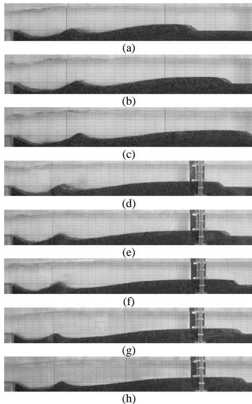
Fig. 16. Bed profile at the end of the bed jet phase for different cycles of run no. 7 (the picture zoom in frames a-c is larger than in frames d-h): (a)  $t = 2801$  s (cycle no. 19); (b)  $t = 5776$  s (cycle no. 32); (c)  $t = 8202$  s (cycle no. 43); (d)  $t = 17662$  s (cycle no. 83); (e)  $t = 20329$  s (cycle no. 93); (f)  $t = 23022$  s (cycle no. 103); (g)  $t = 26031$  s (cycle no. 114); (h)  $t = 27397$  s (cycle no. 119).
