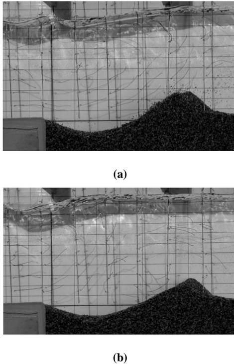
**Fig. 10. Wool-wire flow visualizations for *bed-surface jet* scour hole regime (test no. 14): a)  $t=240$  s (1<sup>st</sup> cycle; bed jet phase); b)  $t=290$  s (1<sup>st</sup> cycle; surface jet phase).**
