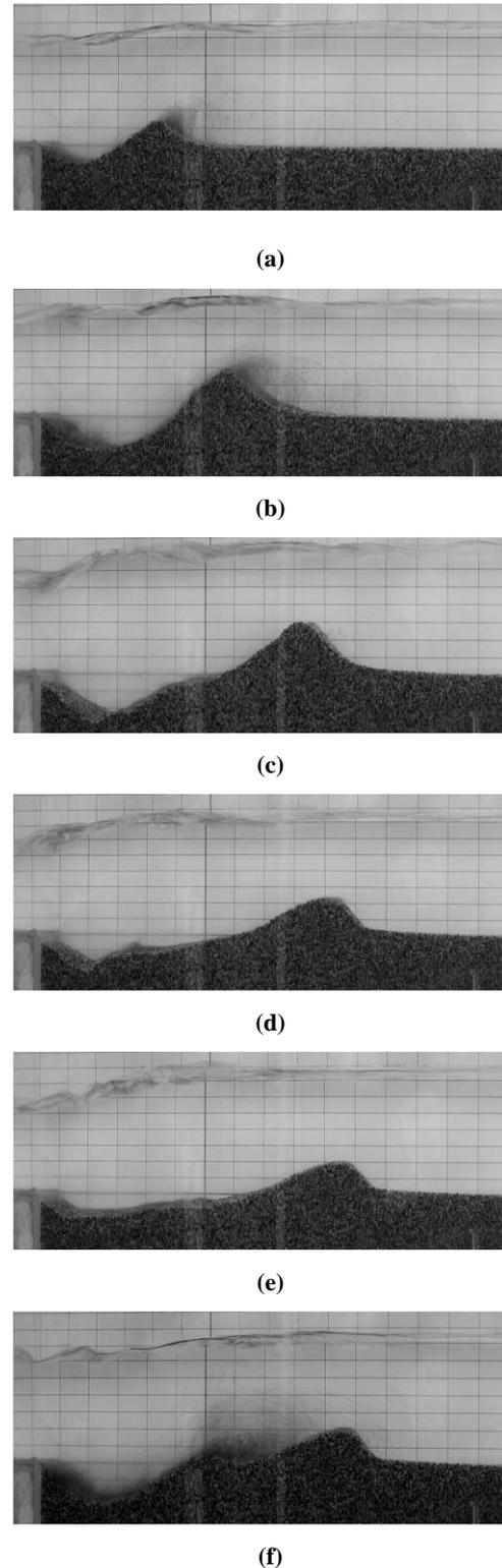
**Fig. 11. Sequence from run no. 7: 1<sup>st</sup> complete cycle and beginning of the 2<sup>nd</sup> bed jet phase. First bed jet phase: a)  $t = 31$  s; b)  $t = 61$  s. First surface jet phase: c)  $t = 92$  s; d)  $t = 122$  s; e)  $t = 153$  s. Second bed jet phase: f)  $t = 164$  s.**
