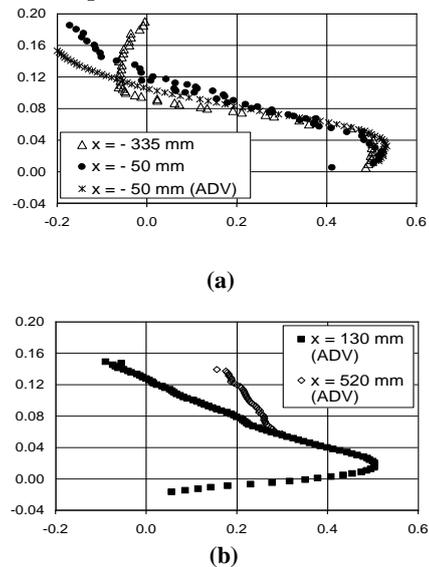
Fig. 8. LDA and ADV vertical profiles of  $u$  (in m/s) vs.  $y$  (in m) at different  $x$  positions for test no. 15: (a)  $x/l = -0.66$  and  $x/l = -0.1$  located above the apron (b)  $x/l = 0.26$  and  $x/l = 1$ , located on scour hole and dune.
