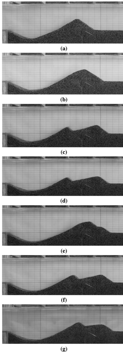
**Fig. 13.** Bed profile at the end of the bed jet phase for different cycles of run no. 9: (a)  $t = 1165$  s (cycle no. 1); (b)  $t = 2400$  s (cycle no. 2); (c)  $t = 7975$  s (cycle no. 3); (d)  $t = 11641$  s (cycle no. 4); (e)  $t = 14700$  s (cycle no. 5); (f)  $t = 21000$  s (cycle no. 6); (g)  $t = 25117$  s (cycle no. 7).
