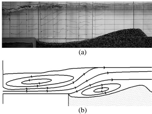
**Fig. 3. Flow visualization and flow-pattern for surface jet scouring regime:**
