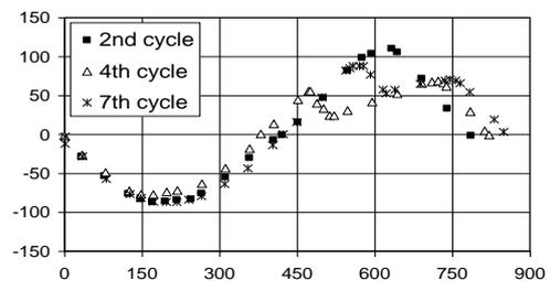
**Fig. 15.** Dimensional bed profiles  $y$  vs.  $x$  (in mm) after the bed jet phase for different cycles of run no. 9. Profiles are carried out for processing frames b, d) and g) of Fig. 13.
