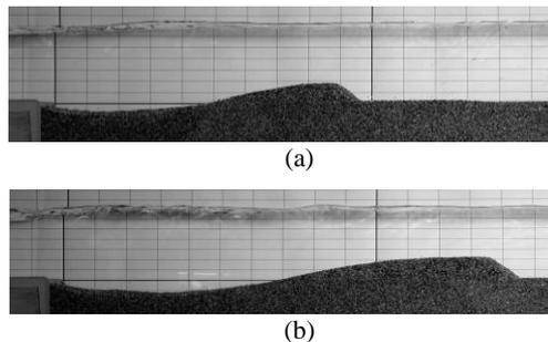
**Fig. 4. Erodible bed profile for test no. 13 (surface jet scouring regime). Images of the bed profile:** (a)  $t = 3600$  s; (b)  $t = 28800$  s.
