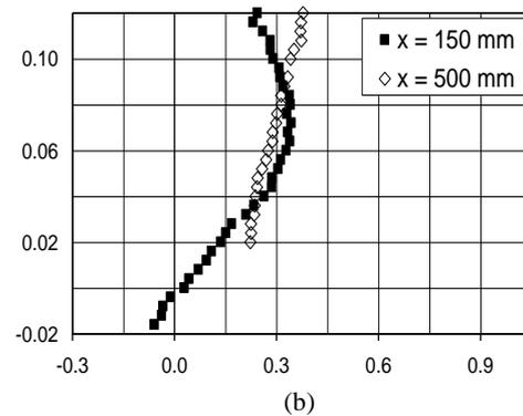
**Fig. 5. LDA vertical profiles of  $u$  (in m/s) vs.  $y$  (in m) at different  $x$  positions for test no. 13:**
