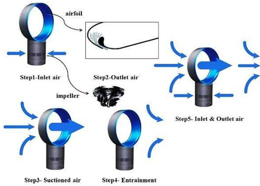
**Fig. 1. Mechanism of entry and exit airflow from bladeless fan.**
