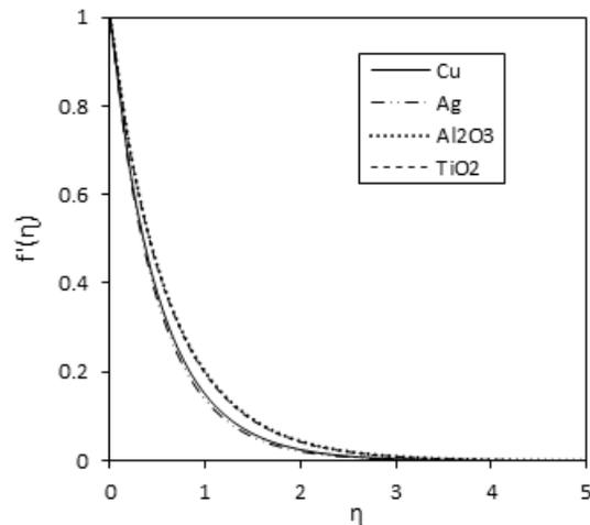
**Fig. 11. Velocity profiles of different types of nanoparticles when  $N_R = 2$ ,  $f_w = 0.2$ ,  $M = 1$ ,  $St = 0.8$  and  $\phi = 0.1$ .**
