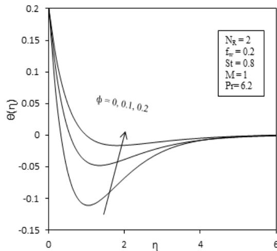
**Fig. 3. Temperature profiles of Cu-water nanofluid with different values of  $\phi$ .**
