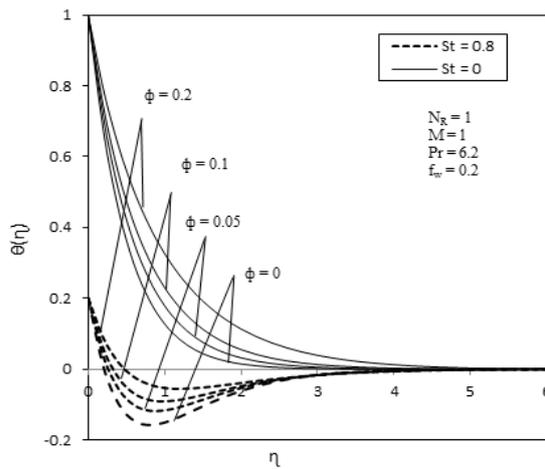
**Fig. 10. Volume fraction effects of Cu-water nanofluid on temperature in stratified and unstratified medium.**
