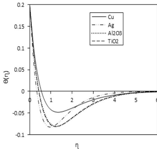
**Fig. 12. Temperature profiles of different types of nanoparticles when  $NR = 2$ ,  $f_w = 0.2$ ,  $M = 1$ ,  $St = 0.8$  and  $\phi = 0.1$ .**
