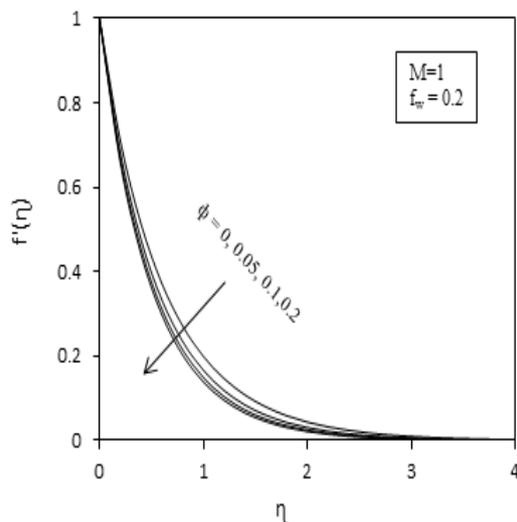
**Fig. 2. Velocity profiles of Cu-water nanofluid for different values of volume fraction parameter  $\phi$ .**
