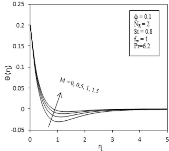
**Fig. 5.** Temperature profiles of Cu-water nanofluid with different values of  $M$ .
