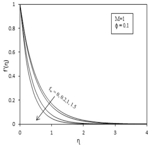
**Fig. 6.** Velocity profiles of Cu-water nanofluid for different values of suction parameter  $f_w$
