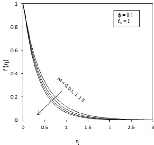
**Fig. 4.** Velocity profiles of Cu-water nanofluid for different values of magnetic parameter  $M$
