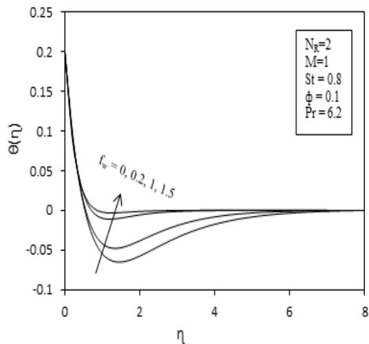
**Fig. 7.** Temperature profiles of Cu-water nanofluid with different values of  $f_w$
