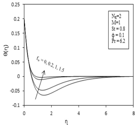
**Fig. 7.** Temperature profiles of Cu-water nanofluid with different values of  $f_w$
