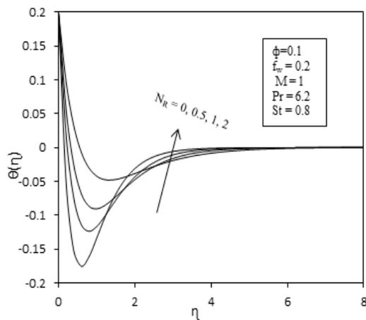
**Fig. 8.** Temperature profiles of Cu-water nanofluid with different values of  $N_R$
