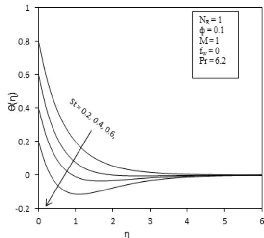
**Fig. 9.** Temperature profiles of Cu-water nanofluid with different values of stratification parameter.
