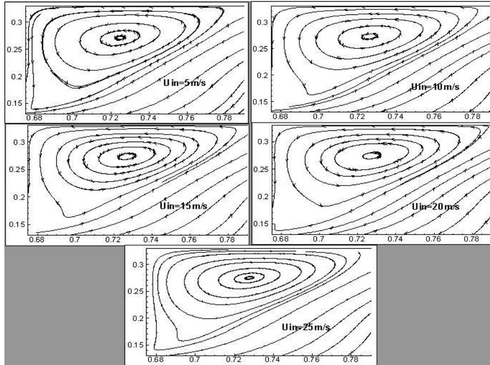
Fig. 5. Vortex formation of vertical limb (Vortex 2)
