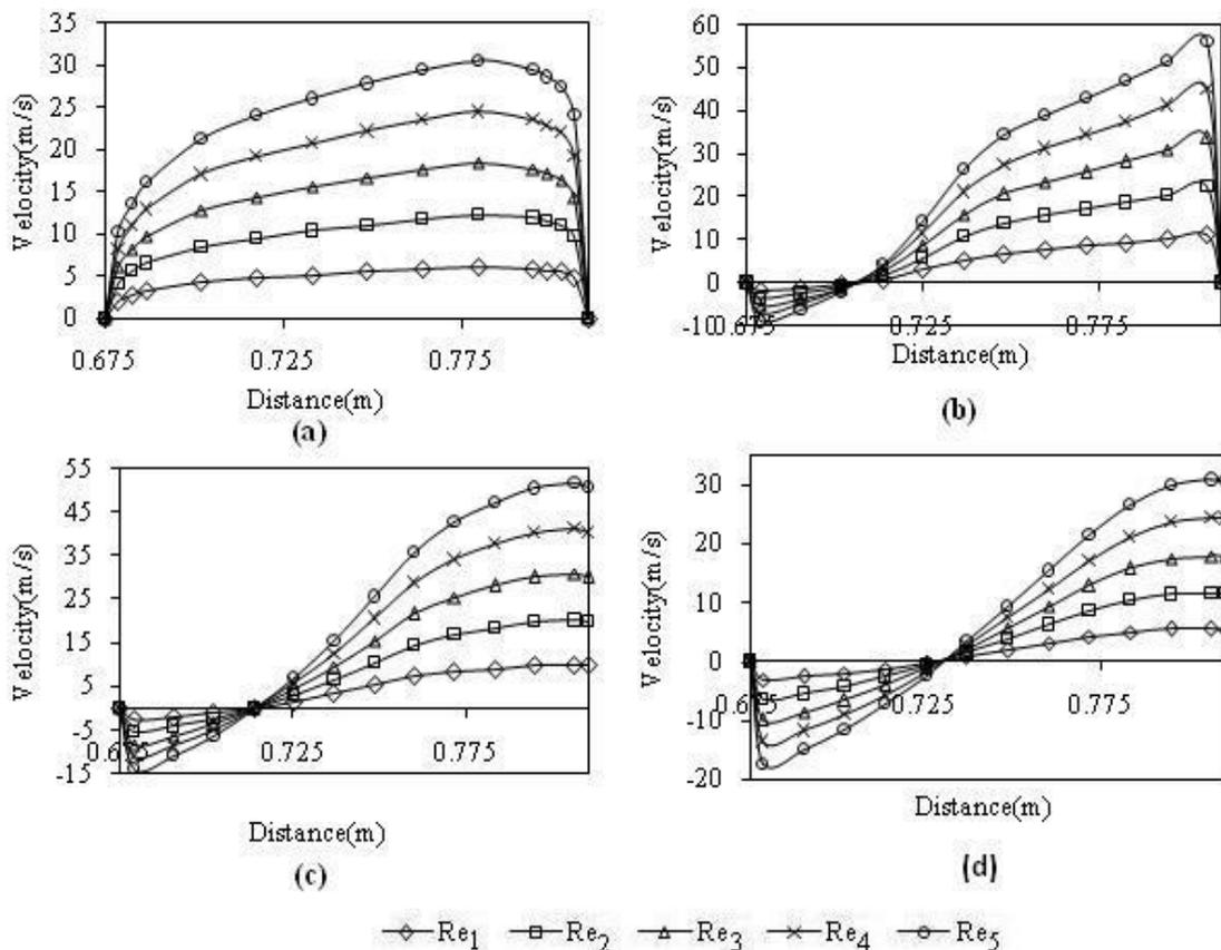
Fig. 4. Velocity profile in the vertical limb at (a)  $Y=0.135$  m, (b)  $Y=0.195$  m, (c)  $Y=0.225$  m, (d)  $Y=0.285$  m
