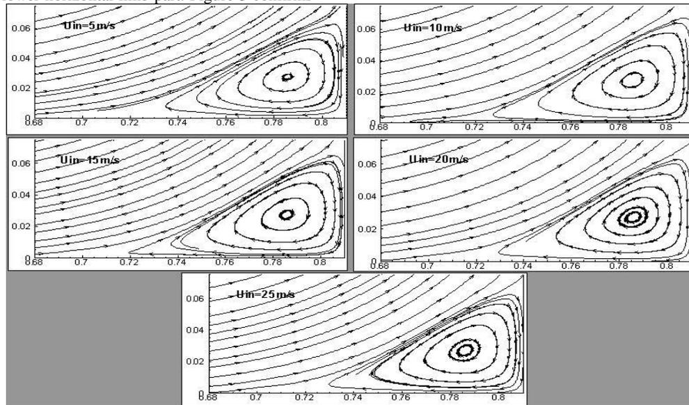
Fig. 3. Vortex formation in the lower Limb (Vortex1)
