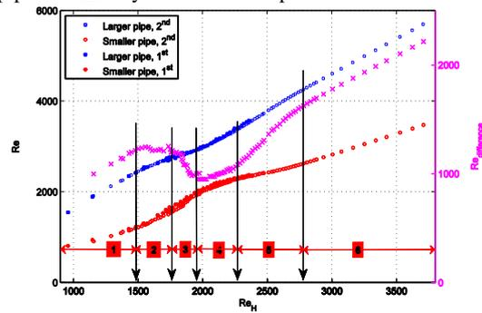
Fig. 4. Reynolds number for the two parallel pipes as a function of  $Re_H$ .
