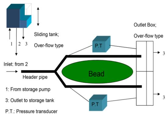
**Fig. 1. Schematic drawing of flow model and experimental setup**
