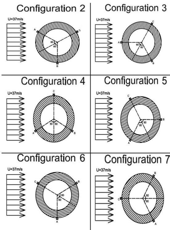
Fig. 1b. Schematic of the model and configurations of plasma actuator.
