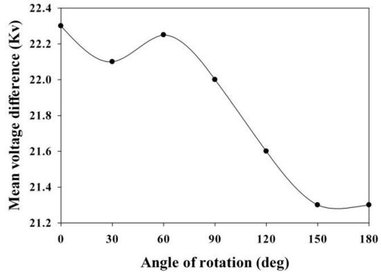
**Fig. 3. The behavior of the mean voltage difference for all configurations of plasma actuator.**
