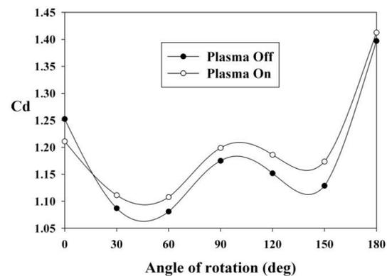
**Fig. 7. Drag coefficient of the cylinder for all configurations of plasma actuator in both plasma on and off conditions.**
