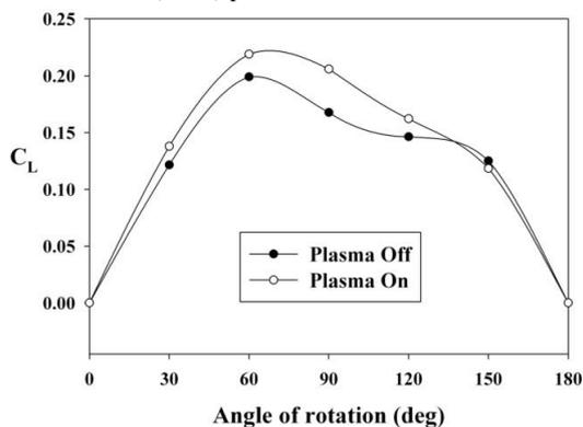
**Fig. 8. Lift coefficient of the cylinder for all configurations of plasma actuator in both plasma on and off conditions.**
