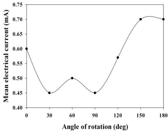
**Fig. 4. The behavior of the mean electrical current for all configurations of plasma actuator.**
