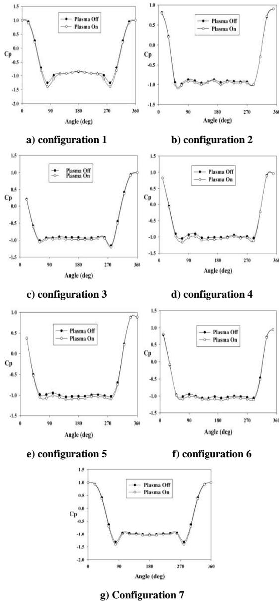
**Fig. 6. Effect of plasma on pressure distribution of the cylinder for configurations 1 to 7.**
