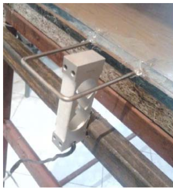
Fig. 2. Configuration of load cell and floating surface.
