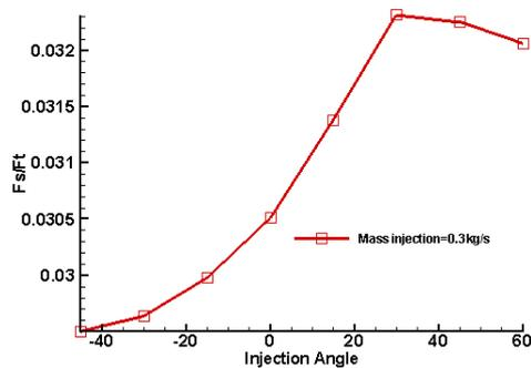
**Fig. 9. Injection angle effect on thrust vector deviation for Freon ( $X_{inj} = 30\%$  Nozzle divergence length).**
