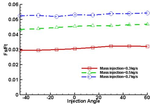
**Fig. 8. Injection angle effect at vary injection flow rate on thrust vector deviation for Freon ( $X_{inj} = 30\%$  Nozzle divergence length).**
