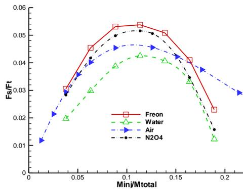
**Fig. 15. Comparison effect of different fluid on thrust vector deviation.**
