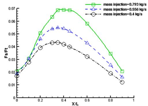
**Fig. 4. Injection position effect for Freon (injection angle=30 degree).**
