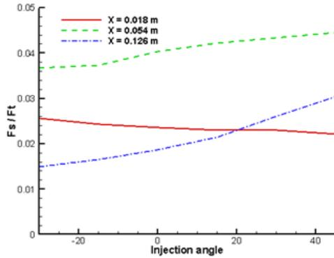
**Fig. 12. Injection angle effect for three injection position, for  $N_2O_4$  fluid and  $m_{inj}=0.5$  kg/s.**
