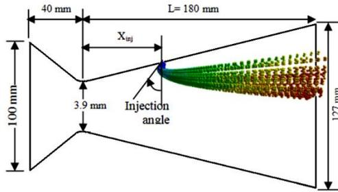
**Fig. 3. Nozzle and injector geometrical parameters.**
