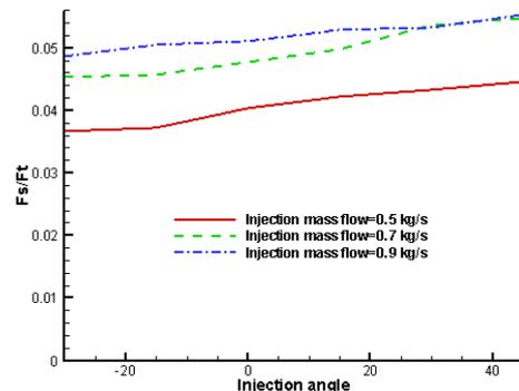
**Fig. 11. Injection angle effect for three injection rate at  $X_{inj}=0.054$  m for  $N_2O_4$ .**
