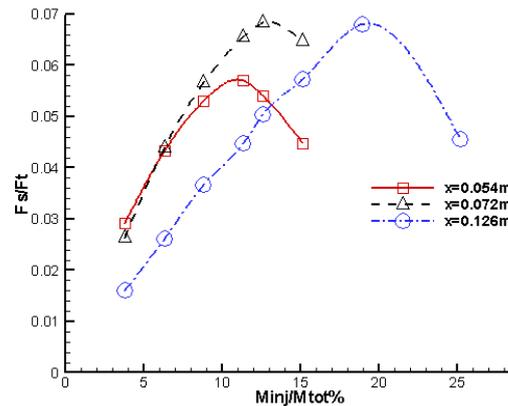
Fig. 7. Thrust vector variation for different injection flow rate for  $N_2O_4$  (Injection angle =30 degree).
