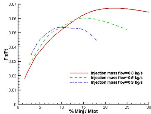
**Fig. 13. effect of total flow rate of main flow on thrust vector deviation for Freon.**
