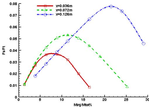
Fig. 6. Injection flow rate effect for Freon (injection angle=30 degree).
