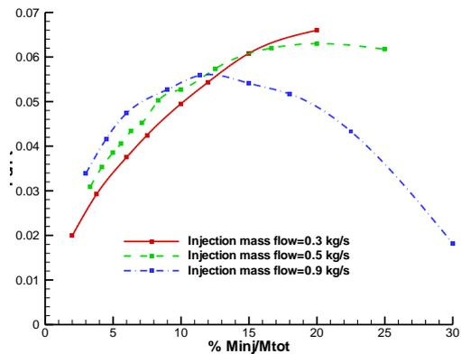
**Fig. 14. Effect of total flow rate of main flow on thrust vector deviation for  $N_2O_4$ .**
