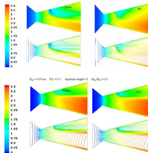
**Fig. 16. Much contour for Freon, air, water and N<sub>2</sub>O<sub>4</sub>.**
