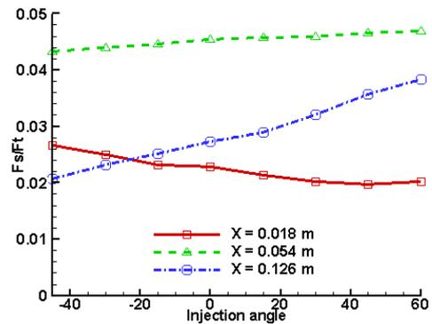
**Fig. 10. Injection angle effect in different injection position for Freon ( $m_{inj}=0.5$  kg/s).**
