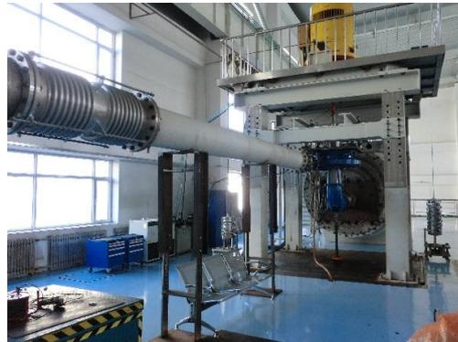
Fig. 1. Pump turbine model test rig installed at HEC, China.
