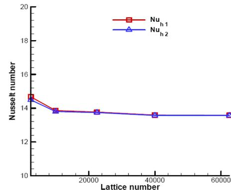
**Fig.4. Effect of the lattice number on Nusselt number for  $A=1$ ,  $Ra = 10^5$ ,  $D = 0.4$  and  $H = 0.05$**
