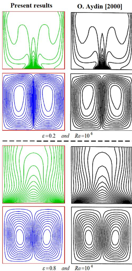
**Fig. 5. Comparison of the present results with O. Aydin [2000] for a centred hot source: isotherms (top) and streamlines (bottom).**
