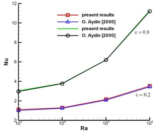
**Fig. 6. Comparison of the average Nusselt number versus Rayleigh along hot wall for a centred hot source of length  $\epsilon = 0.2$  and  $0.8$  with previous findings.**
