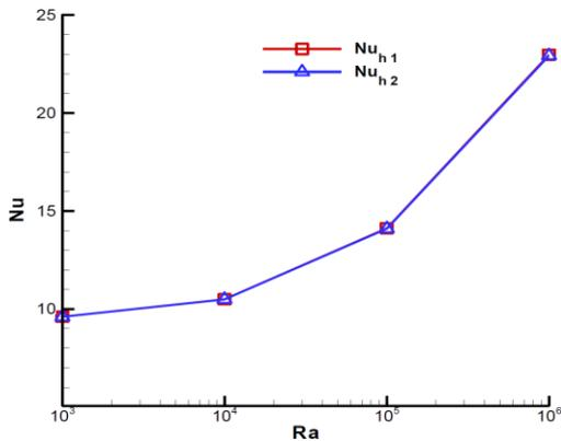
**Fig. 11.** Variation of the average Nusselt number along horizontal hot upper wall of heat blocks  $S_1$  and  $S_2$  for various Rayleigh number with  $A = 1$ ,  $D = 0.6$  and  $H = 0.05$ .
