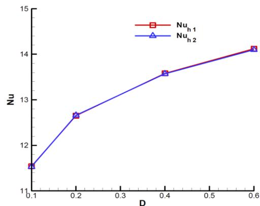
**Fig.12.** Variation of the average Nusselt number along horizontal hot upper wall of heat blocks  $S_1$  and  $S_2$  for various blocks spacing with  $A = 1$ ,  $Ra = 10^5$  and  $H = 0.05$
