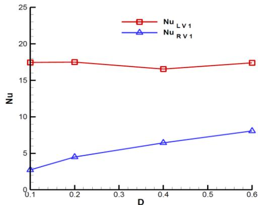
**Fig. 16.** Variation of the average Nusselt number along vertical hot walls of heat block  $S_1$  for various blocks spacing with A = 1, Ra =  $10^5$  and H = 0.05.
