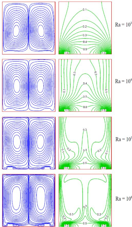
**Fig. 7. Streamlines (left) and isotherms (right) vs. Rayleigh number with  $A = 1$ ,  $H = 0.05$  and  $D = 0.6$ .**
