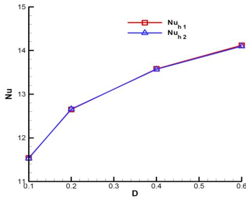
**Fig.12.** Variation of the average Nusselt number along horizontal hot upper wall of heat blocks  $S_1$  and  $S_2$  for various blocks spacing with  $A = 1$ ,  $Ra = 10^5$  and  $H = 0.05$
