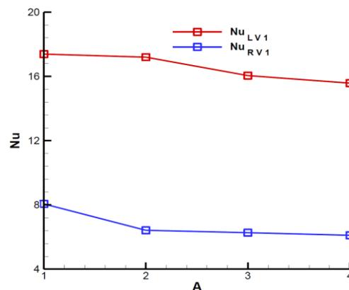
**Fig.18.** Variation of the average Nusselt number along vertical hot walls of heat block  $S_1$  for various aspect ratio of the enclosure with Ra =  $10^5$ , D = 0.6 and H = 0.05.
