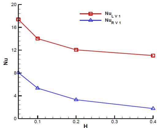
**Fig. 17.** Variation of the average Nusselt number along vertical hot walls of heat block  $S_1$  for various block height with A = 1, Ra =  $10^5$  and D = 0.6
