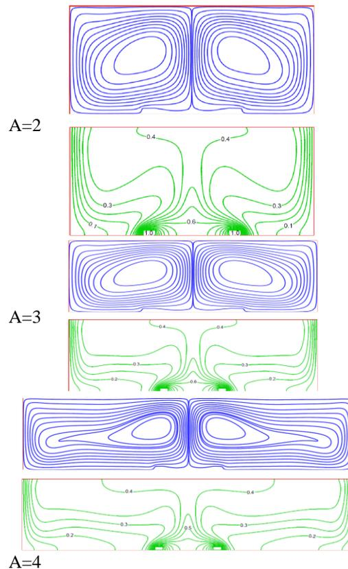
**Fig. 10. Streamlines (top) and isotherms (bottom) vs. aspect ratio of the enclosure With  $Ra = 10^5, D = 0.6$  and  $H = 0.05$**
