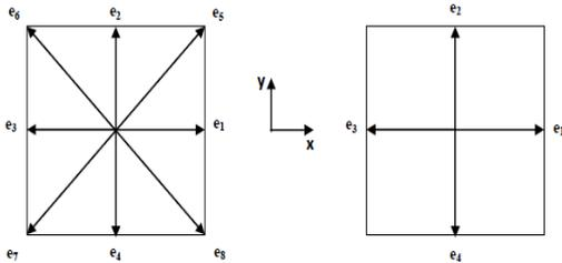
**Fig. 2. Lattice structure for two dimensional with D2Q4-D2Q9 models.**
