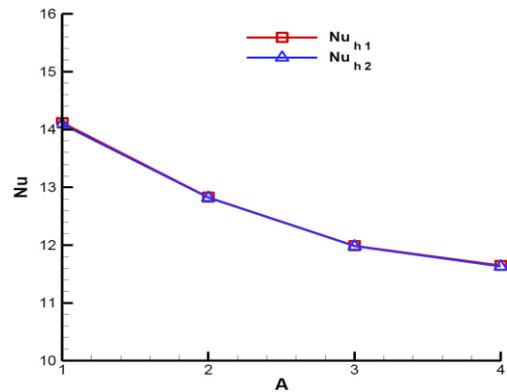
**Fig. 14.** Variation of the average Nusselt number along horizontal hot upper wall of heat blocks  $S_1$  and  $S_2$  for various aspect ratio of the enclosure with  $Ra = 10^5$ ,  $D = 0.6$  and  $H = 0.05$ .
