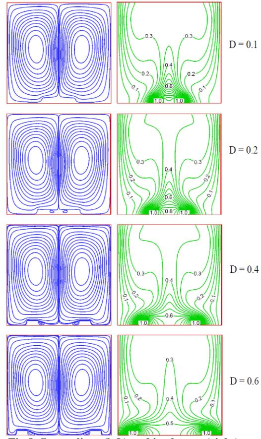
**Fig.8. Streamlines (left) and isotherms (right) vs. spacing between heat blocks with  $A = 1$ ,  $Ra = 10^5$  and  $H = 0.05$ .**
