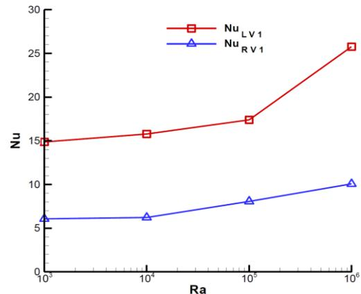
**Fig.15.** Variation of the average Nusselt number along vertical hot walls of heat block  $S_1$  for various Rayleigh number with  $A = 1$ ,  $D = 0.6$  and  $H = 0.05$ .
