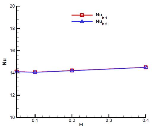
**Fig. 13.** Variation of the average Nusselt number along horizontal hot upper wall of heat blocks  $S_1$  and  $S_2$  for various block height with  $A = 1$ ,  $Ra = 10^5$  and  $D = 0.6$ .
