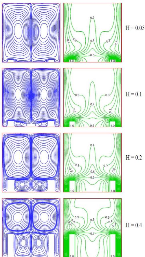
**Fig. 9. Streamlines (left) and isotherms (right) vs. height of heat sources with  $A = 1$ ,  $Ra = 10^5$  and  $D = 0.6$**
