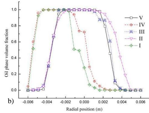
**Fig. 6. Oil phase volume fraction contours and radial profiles. a) oil phase volume fraction contour; b) radial profiles of oil phase volume fraction at different cross-section.  $v_{so}=0.15$  m/s and  $v_{sw}=0.15$  m/s, downflow.**
