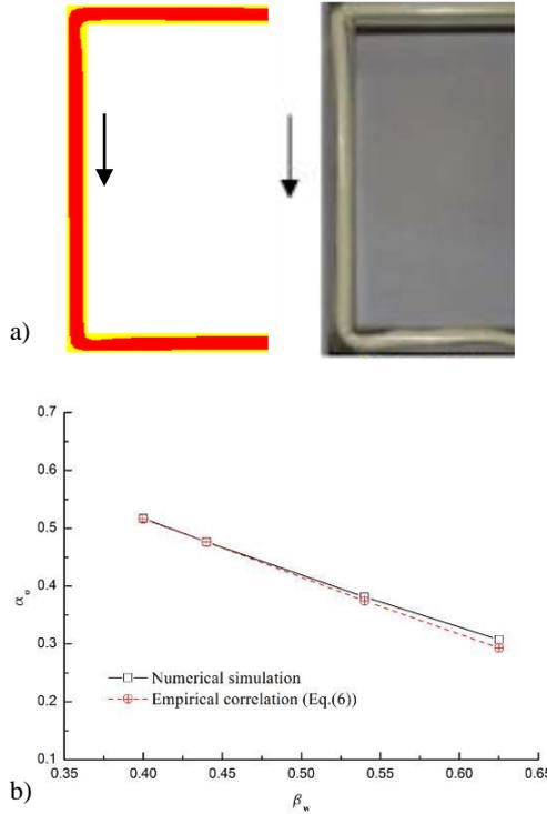
**Fig. 5. Comparison with experiment and empirical correlation. a) numerical and experimental contour during core annular downflow through the U-bend; oil, water. b) numerical results and empirical correlation.  $v_{so}=0.4-0.6$  m/s and  $v_{sw}=0.6-1.0$  m/s, downflow.**
