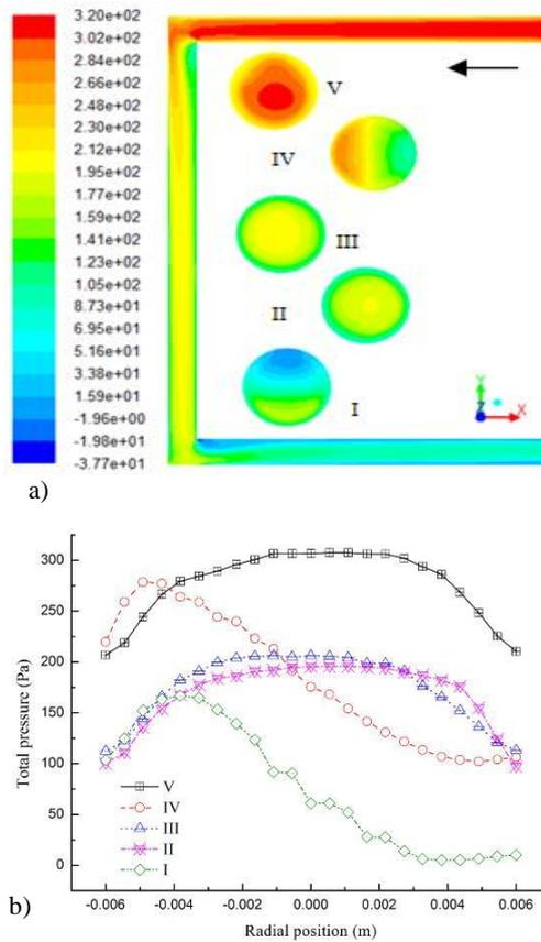
**Fig. 7. Pressure contours and radial profiles. a) total pressure contour; b) pressure radial profiles at different cross-section.  $v_{so}=0.15$  m/s and  $v_{sw}=0.15$  m/s, downflow.**
