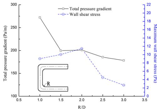
**Fig. 15. Total pressure gradient and maximum wall shear stress as a function of  $R/D$ .**
