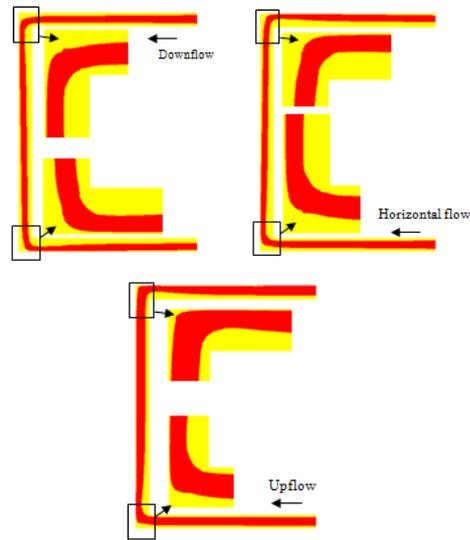
**Fig. 12. Oil phase distribution comparison of different flow directions.**
