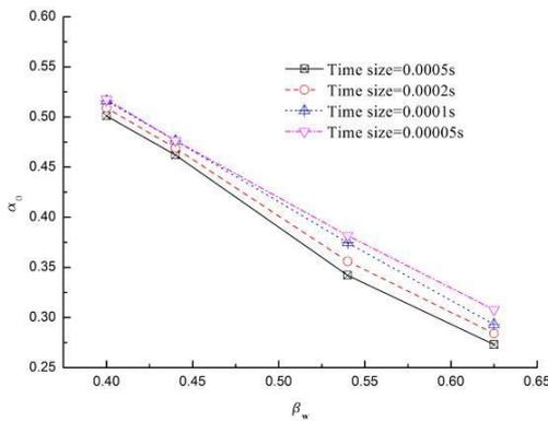
**Fig. 4. The comparison of average of oil volume fraction under different time step size and discretized scheme.  $v_{so}=0.4-0.6$  m/s and  $v_{sw}=0.6-1.0$  m/s, downflow.**
