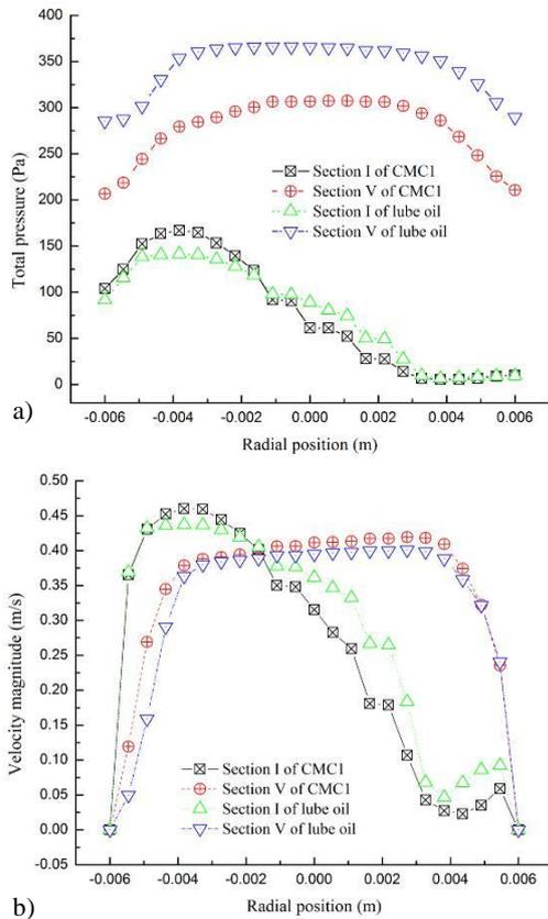
**Fig. 11. Flow parameters comparison of Newtonian oil and non-Newtonian oil.**
