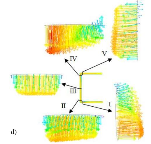
**Fig. 8. Velocity contours, radial profiles and velocity vector. a) velocity magnitude contour; b) velocity radial profiles at different cross-section; c) velocity vector of longitudinal section; d) velocity vector of cross-sections.  $v_{so}=0.15$  m/s and  $v_{sw}=0.15$  m/s, downflow.**
