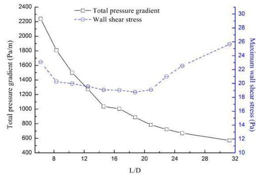
**Fig. 13. Total pressure gradient and maximum wall shear stress as a function of L/D.**
