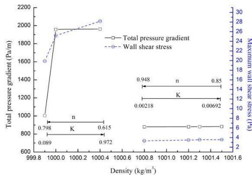
**Fig. 9. Variation of total pressure gradient and maximum wall shear stress with the non-Newtonian oil properties.**
