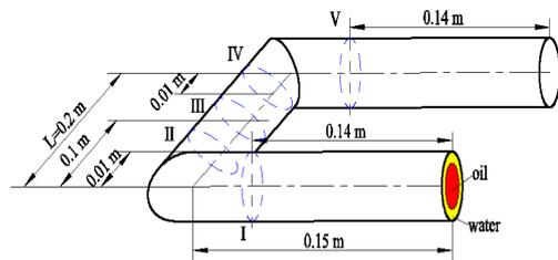
Fig. 1. Geometry of computational domain.
