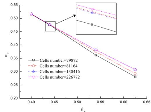
Fig. 3. The comparison of average of oil volume fraction under different cells number.  $v_{so}=0.4-0.6$  m/s and  $v_{sw}=0.6-1.0$  m/s, downflow.
