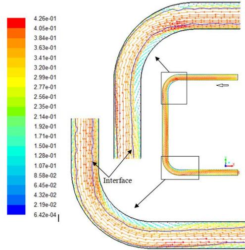
**Fig. 16. Vector and interface of non-Newtonian oil and water flow in the rounding  $\Gamma$ -bend.**
