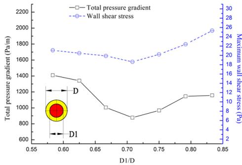
**Fig. 14. Total pressure gradient and maximum wall shear stress as a function of  $D1/D$ .**
