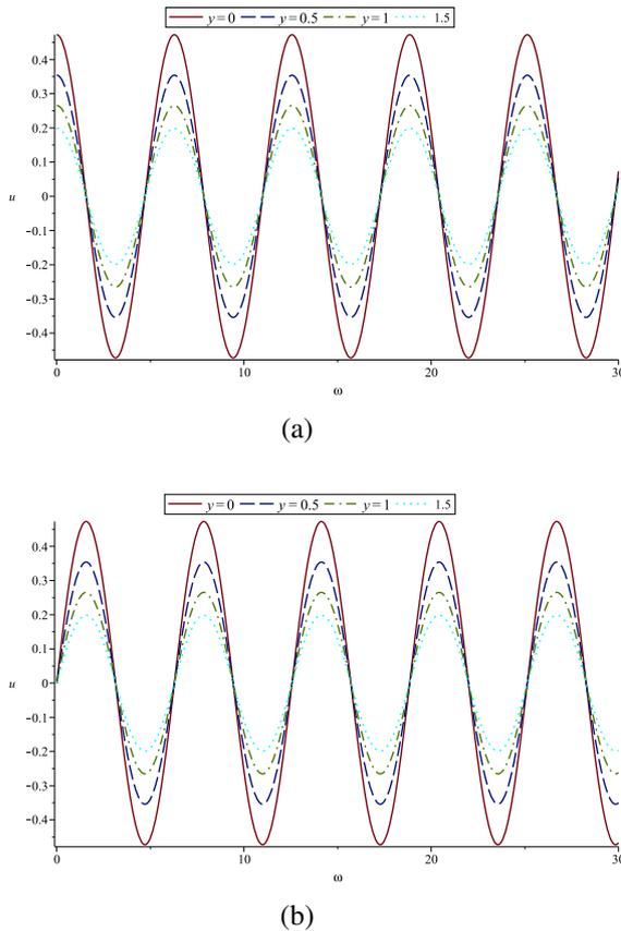
**Fig. 8. Frequency series of the flow velocity with different values of the distances from the plate  $y$  when  $\beta = 1.5$ ,  $\beta_* = 0.5$ ,  $M_* = 1$ ,  $\phi_* = 0.5$ ,  $t = 1$ ,  $\mu_* = 0.5$ ,  $\alpha_* = 0.5$  are fixed (a) Cosine oscillation and (b) Sine oscillation**
