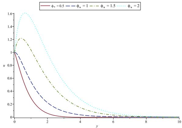
**Fig. 4. Profiles of the flow velocity with different values of the porosity of the porous medium parameter  $\phi_*$  when  $\beta = 1.5, \beta_* = 1, M_* = 0.5, k = 1, \mu_* = 0.5, \alpha_* = 0.5$  are fixed**
