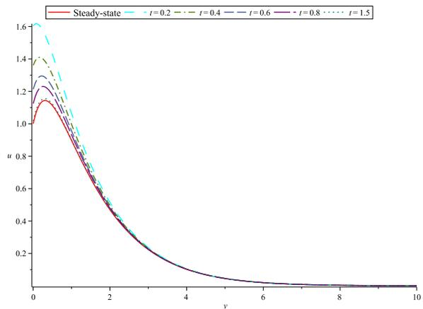
**Fig. 5. Profiles of the starting and steady-state flow velocity with different values of the time  $t$  when when  $\omega = 0.5, k = 1, \beta_* = 2.5, \beta = 1.5, M_* = 0.5, \phi_* = 1, \mu_* = 0.5, \alpha_* = 0.5$  are fixed**
