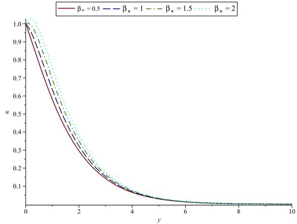
**Fig. 3. Profiles of the flow velocity with different values of the material parameter  $\beta_*$  when  $\beta = 1, M_* = 1, \phi_* = 0.5, k = 1, \mu_* = 0.5, \alpha_* = 0.5$  are fixed**
