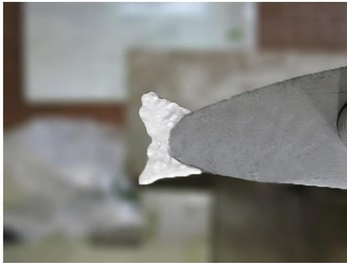
**Fig.3. Foam glaze-ice attached on the model.**
