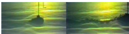
**Fig. 10. Flow around the body in the recirculating mode with Fr=1.0. For the case on the right, some dye was injected over the body (with some small scale turbulence probably due to it being slightly buoyant) to show the flow more clearly.**
