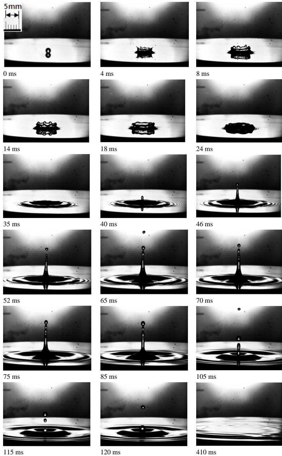
**Fig. 6.** Behavior of an impacting droplet onto a liquid film, for the case of  $h = 10$  mm,  $V=2.75$  m/s.
