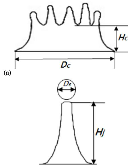
Fig. 2. Schematic of typical droplet behaviors after impact: (a) crown formation, and (b) central jet and secondary drop formation.
