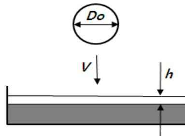
Fig. 1. Impacting droplet onto a liquid film.
