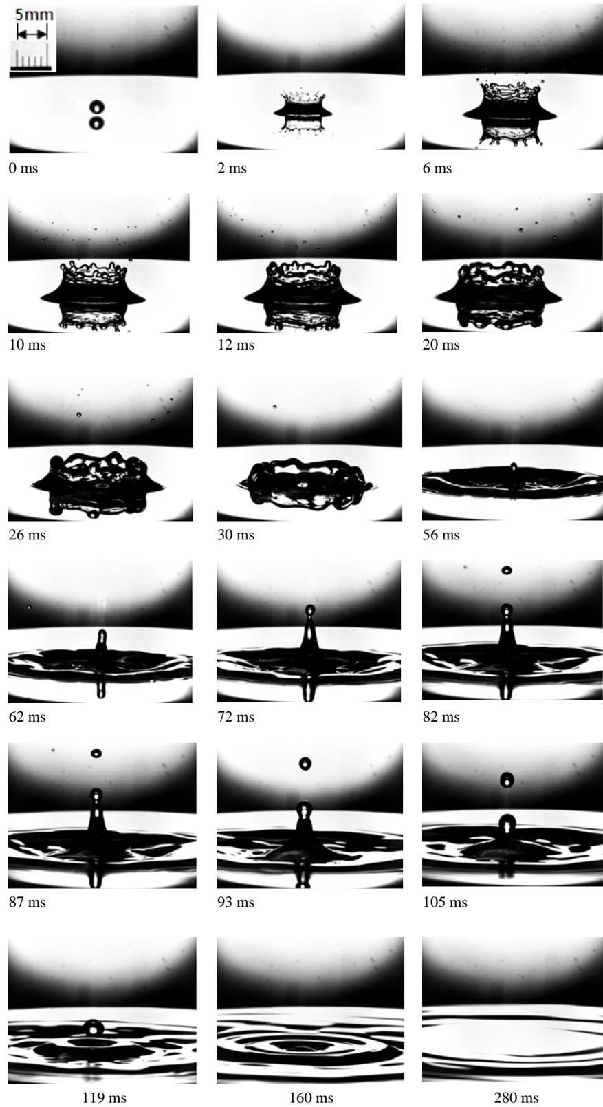
Fig. 5. Behavior of an impacting droplet onto a liquid film, for the case of  $h = 2$  mm,  $V=4.1$  m/s.
