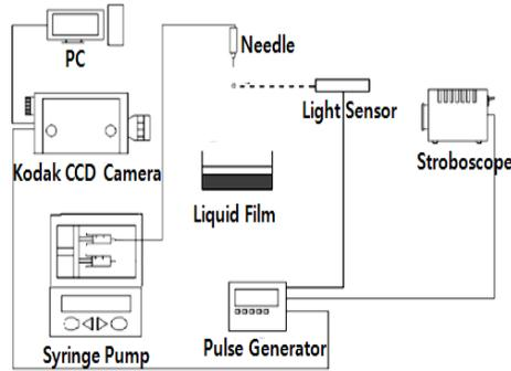
**Fig. 3. A schematic diagram of the experimental setup.**
