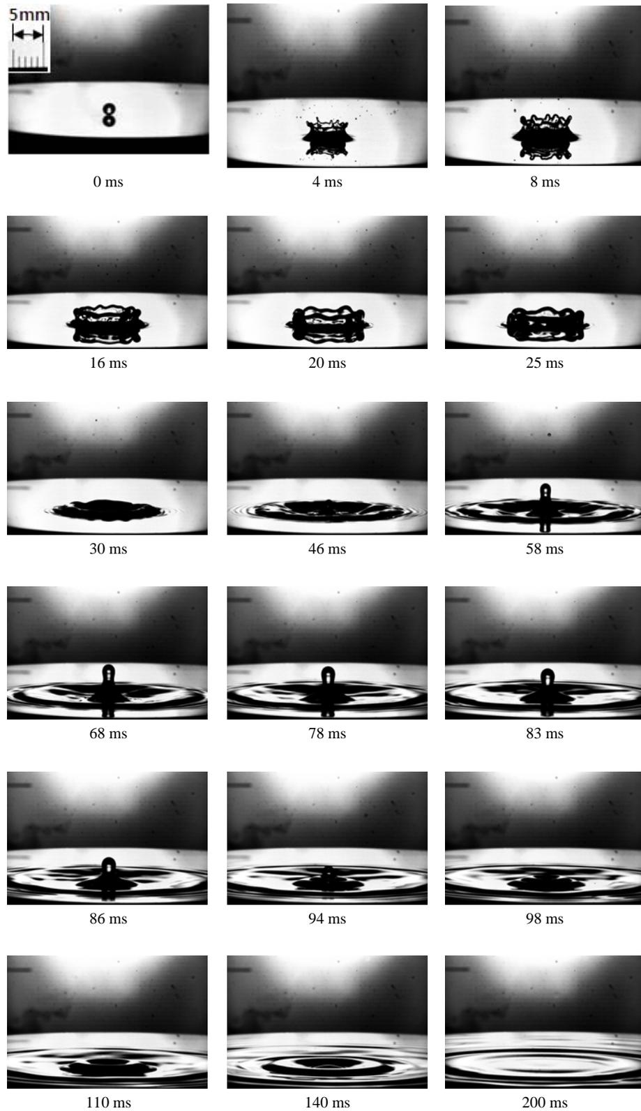
**Fig. 4.** Behavior of an impacting droplet onto a liquid film, for the case of  $h = 2$  mm,  $V = 2.75$  m/s.
