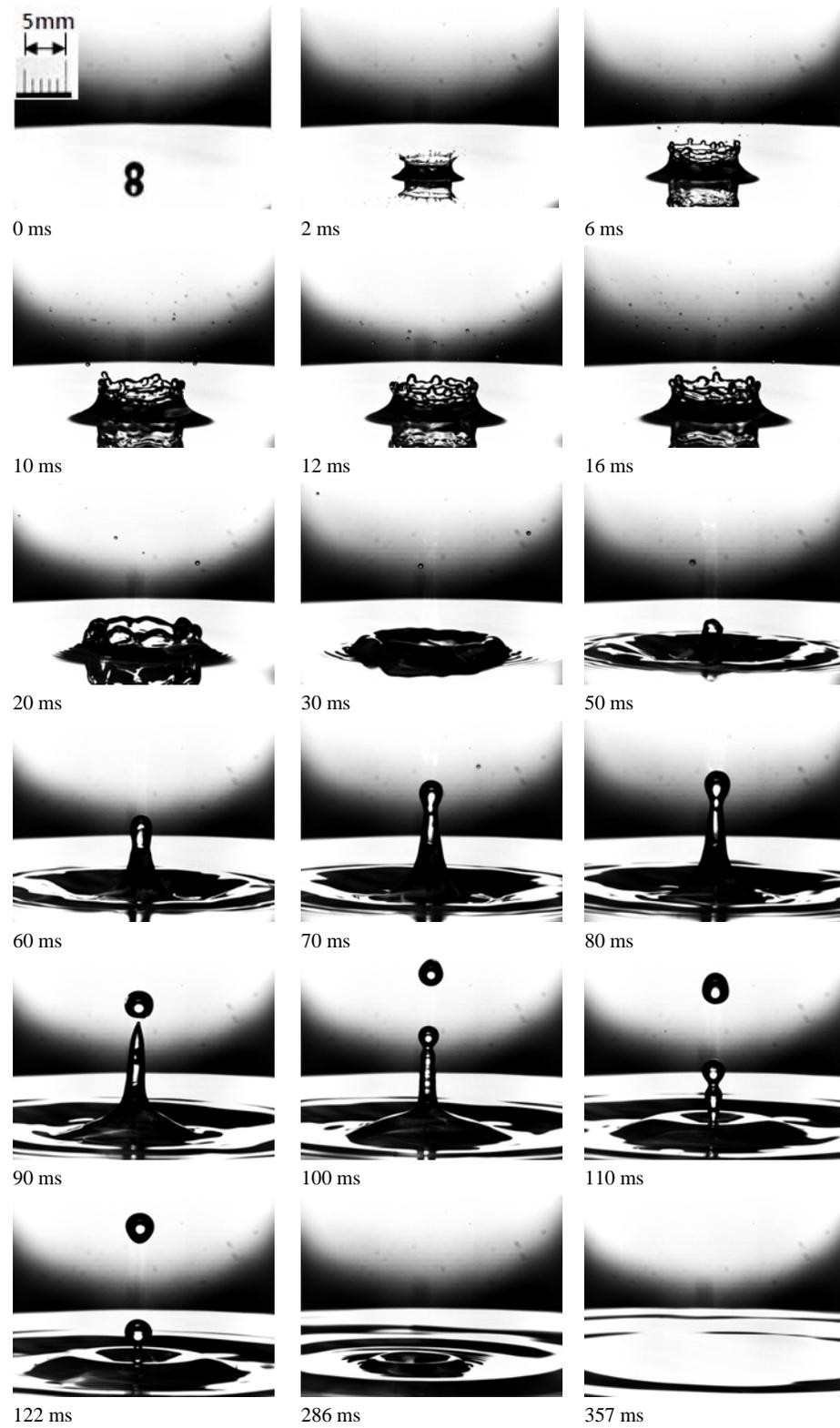
Fig. 7. Behavior of an impacting droplet onto a liquid film, for the case of  $h = 10$  mm,  $V=4.1$  m/s.
