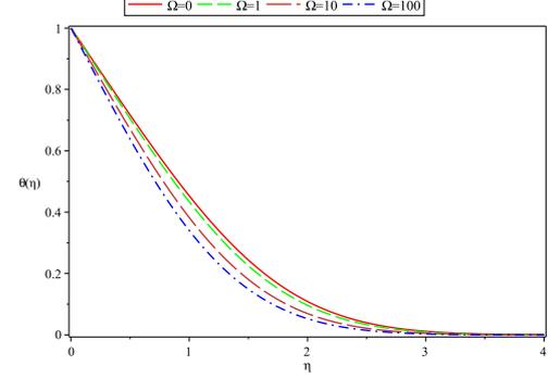
**Fig. 10.** Temperature profiles  $\theta(\eta)$  for  $Pr = 1, M = f_w = \lambda = 0$  and various parameters  $\Omega$ .
