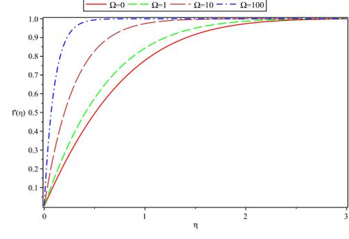
**Fig. 9.** Non-dimensional velocity profiles  $f'(\eta)$  for  $Pr = 1, M = f_w = \lambda = 0$  and various parameters  $\Omega$ .
