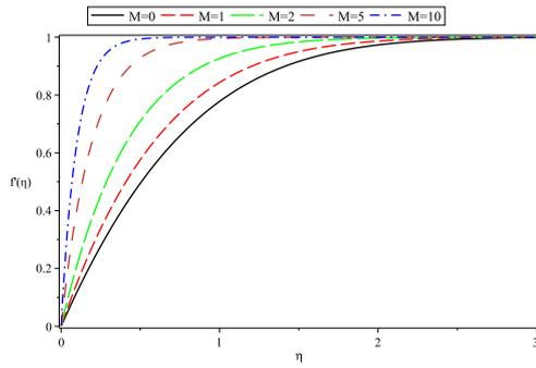
**Fig. 3.** Non-dimensional velocity profiles  $f'(\eta)$  for  $f_w = 0, Pr = 1, \lambda = \Omega = 0$  and various parameters  $M$ .
