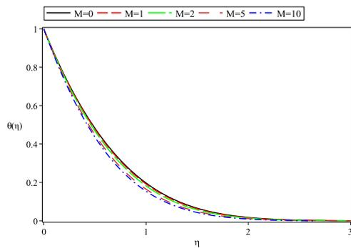
**Fig. 6.** Temperature profiles  $\theta(\eta)$  for  $f_w = 1, Pr = 1, \lambda = \Omega = 0$  and various parameters  $M$ .
