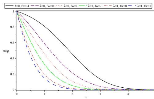
**Fig. 15.** The temperature profiles  $\theta(\eta)$  for  $\Omega = M = 0, Pr = 1, \lambda = 0, 1$  and  $f_w = -1, 0, 1$ .
