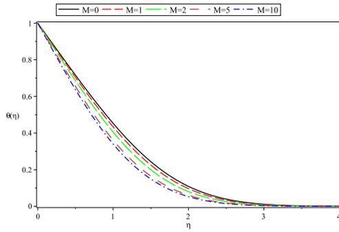
**Fig. 4.** Temperature profiles  $\theta(\eta)$  for  $f_w = 0, Pr = 1, \lambda = \Omega = 0$  and various parameters  $M$ .
