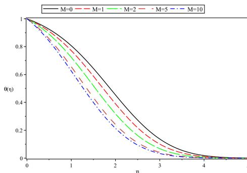
**Fig. 2. The temperature profiles  $\theta(\eta)$  for  $f_w = -1, Pr = 1, \lambda = \Omega = 0$  and various parameters  $M$ .**
