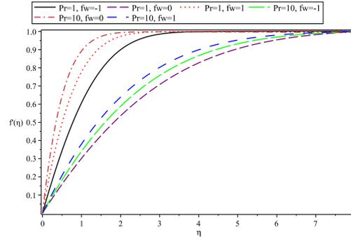
**Fig. 13.** Non-dimensional velocity profiles  $f'(\eta)$  for  $\lambda = \Omega = M = 0, Pr = 1, 10$  and  $f_w = -1, 0, 1$ .
