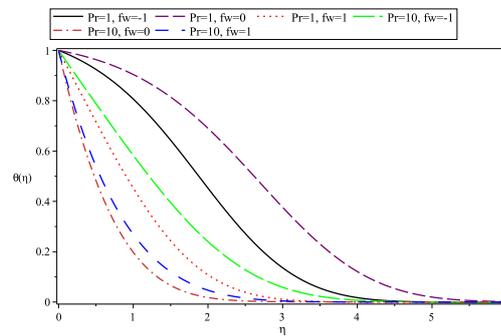
**Fig. 14.** Temperature profiles  $\theta(\eta)$  for  $\lambda = \Omega = M = 0, Pr = 1, 10$  and  $f_w = -1, 0, 1$ .
