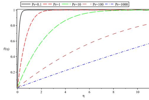
**Fig. 7.** Non-dimensional velocity profiles  $f'(\eta)$  for  $M = f_w = \lambda = \Omega = 0$  and various parameters  $Pr$ .
