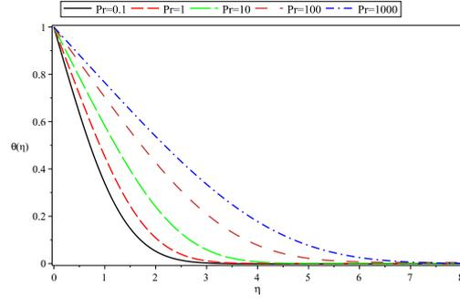
**Fig. 8.** Temperature profiles  $\theta(\eta)$  for  $M = f_w = \lambda = \Omega = 0$  and various parameters  $Pr$ .
