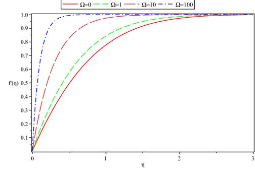
**Fig. 9.** Non-dimensional velocity profiles  $f'(\eta)$  for  $Pr = 1, M = f_w = \lambda = 0$  and various parameters  $\Omega$ .
