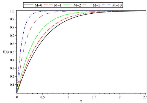
**Fig. 5.** Non-dimensional velocity profiles  $f'(\eta)$  for  $f_w = 1, Pr = 1, \lambda = \Omega = 0$  and various parameters  $M$ .
