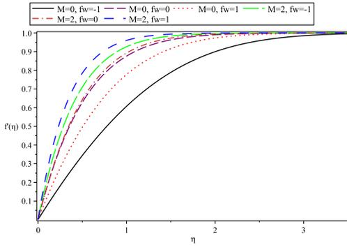
**Fig. 11.** Non-dimensional velocity profiles  $f'(\eta)$  for  $Pr = 1, \lambda = \Omega = 0, M = 0, 2$  and  $f_w = -1, 0, 1$ .
