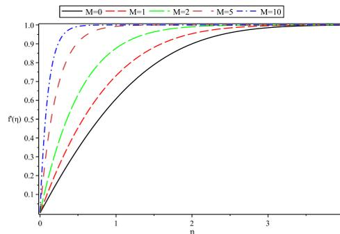
**Fig. 1. The non-dimensional velocity profiles  $f'(\eta)$  for  $f_w = -1, Pr = 1, \lambda = \Omega = 0$  and various parameters  $M$ .**
