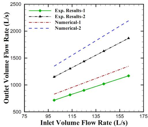
Fig. 13. Comparison of experimental and numerical results of flow increase curve for fan.
