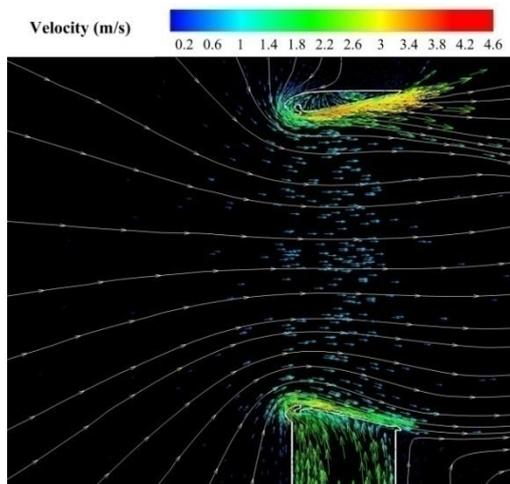
Fig. 12. Velocity vectors of the exit flow for inlet flow rate of 50L/s.
