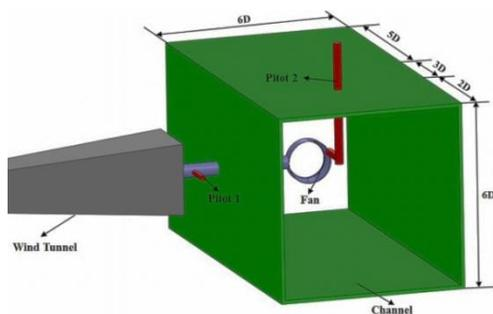
**Fig. 10. Output flow measurement scheme.**
