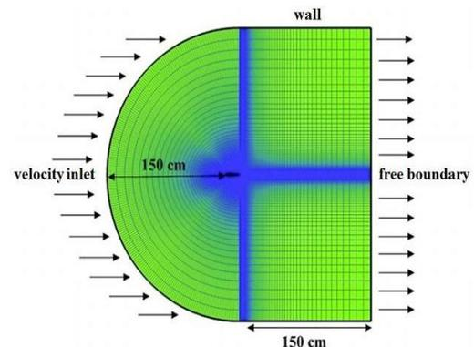
Fig. 5. 2D modeling, boundary conditions, and mesh generation for NACA 0012 airfoil.
