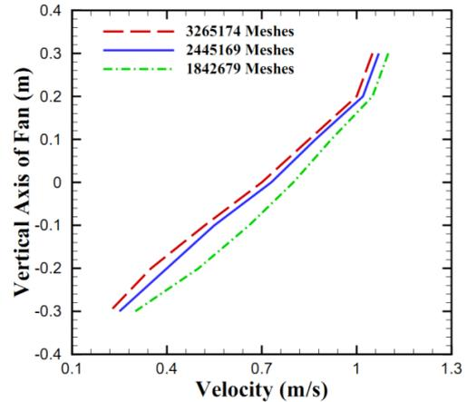
Fig. 4. Velocity profile at 50cm downstream for flow rate of 50L/s.
