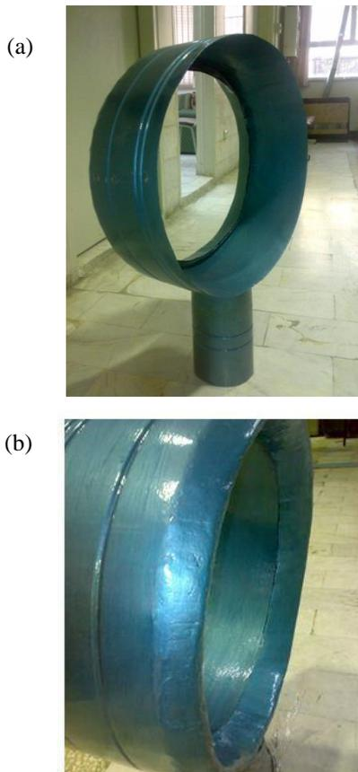
**Fig. 7. a) Constructed Bladeless fan with 60cm diameter. b) Backside of the fan (upstream).**
