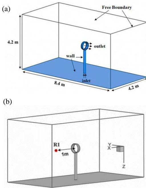
Fig. 3. a) 3D modeling of the fan in a cubic room, b) Sound receiver location.
