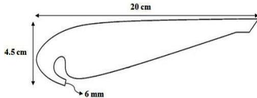
Fig. 2. Designed cross section of the fan.
