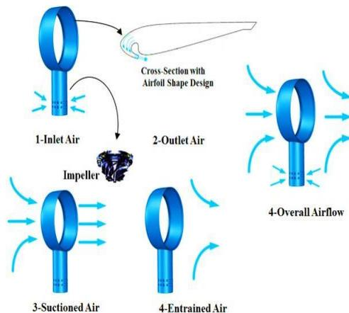
Fig. 1. Schematic of entry and exit airflow through Bladeless Fan.
