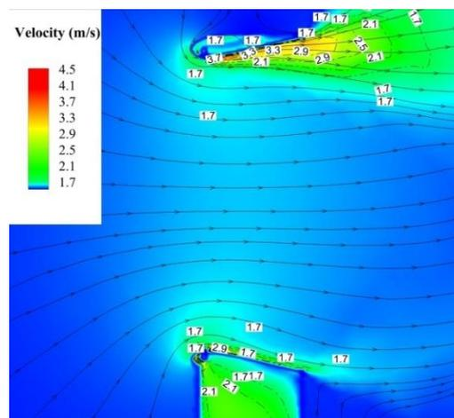
**Fig. 11. Velocity contour in the middle section of fan.**
