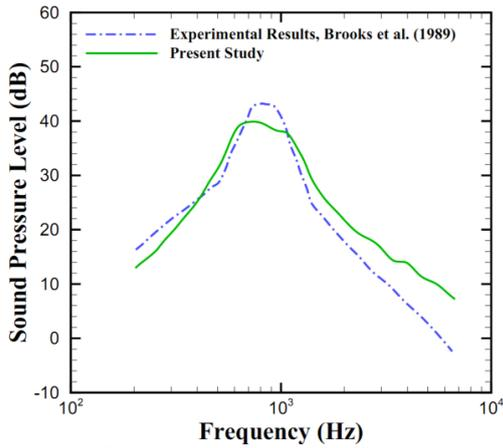
**Fig. 6. Comparison of experimental data and numerical results of produced sound by NACA 0012 airfoil.**
