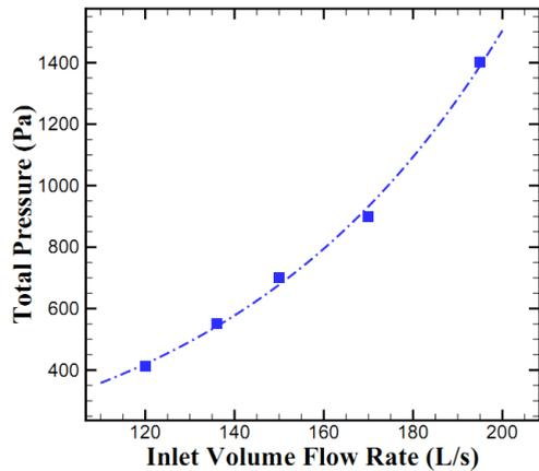
**Fig. 9. Experimental performance curve of the fan.**
