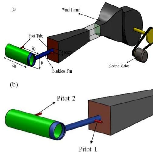
**Fig. 8. a) Illustration of the experimental setup, b) Illustration depicting pitot tubes No. 1 and 2 locations.**
