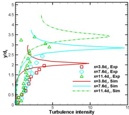
**Fig. 8. Turbulence intensity distributions corresponding at different axial positions for Case 2.**
