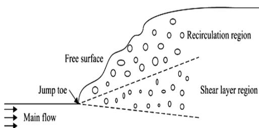
**Fig. 1. Schematic of air entrainment for hydraulic jump flows.**
