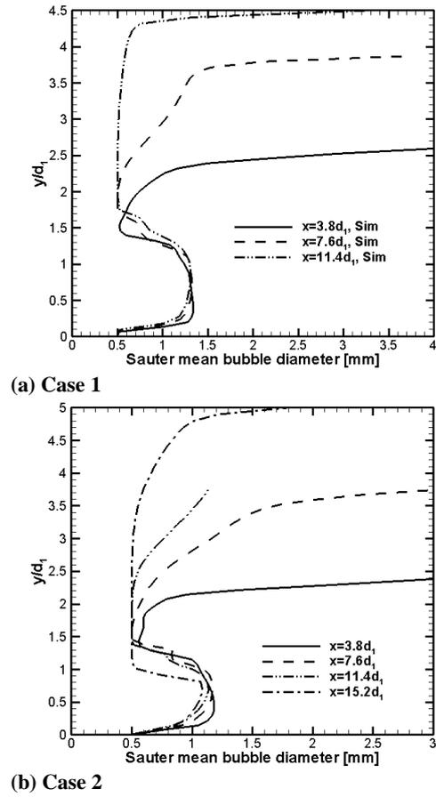
**Fig. 7. Sauter mean bubble diameter distributions corresponding at different axial positions.**
