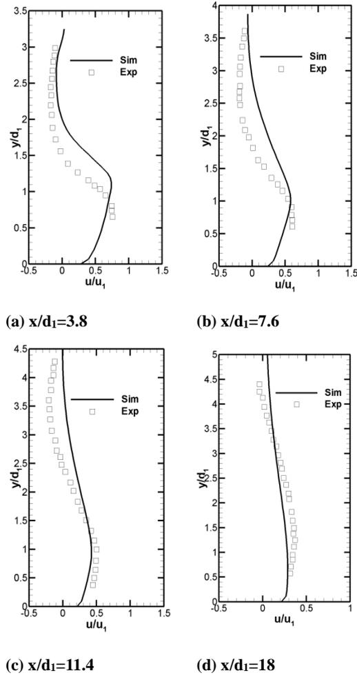
**Fig. 4. Comparison of dimensionless water velocity profile corresponding at different axial positions downstream gas entrainment point for Case 1 with experimental data.**
