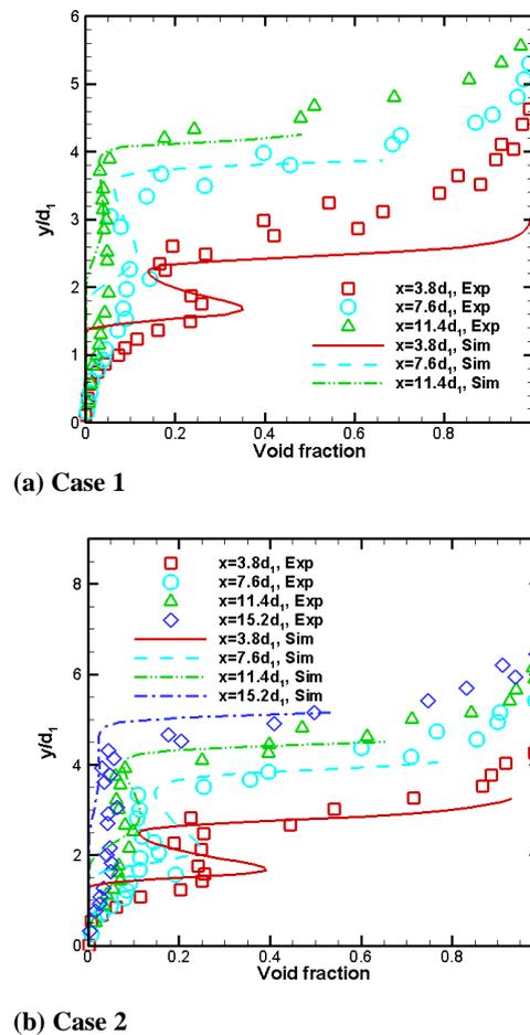
**Fig. 5. Radial void fraction distribution corresponding at different axial positions.**
