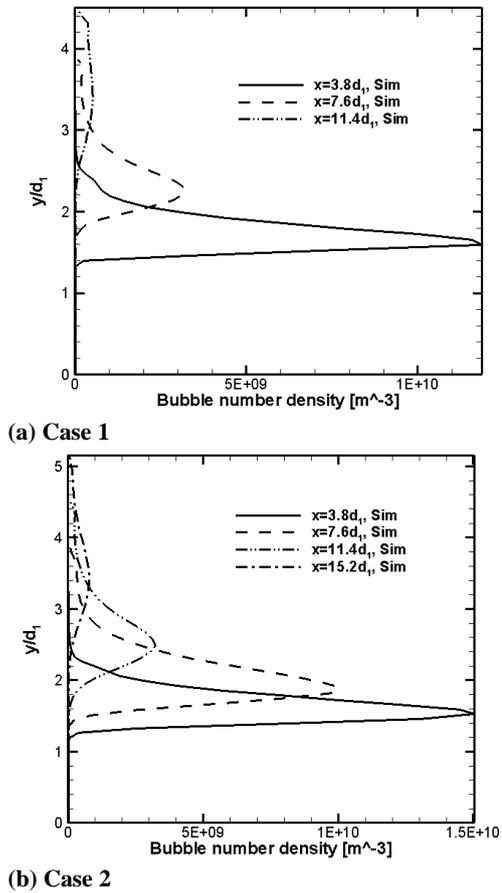
**Fig. 6. Dimensionless bubble number density distributions corresponding at different axial positions.**
