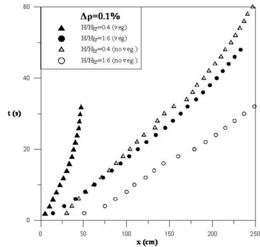
Fig. 3. Effect of relative depth  $H/H_{tr}$  on the motion of gravity current for vegetated and non-vegetated bed.
