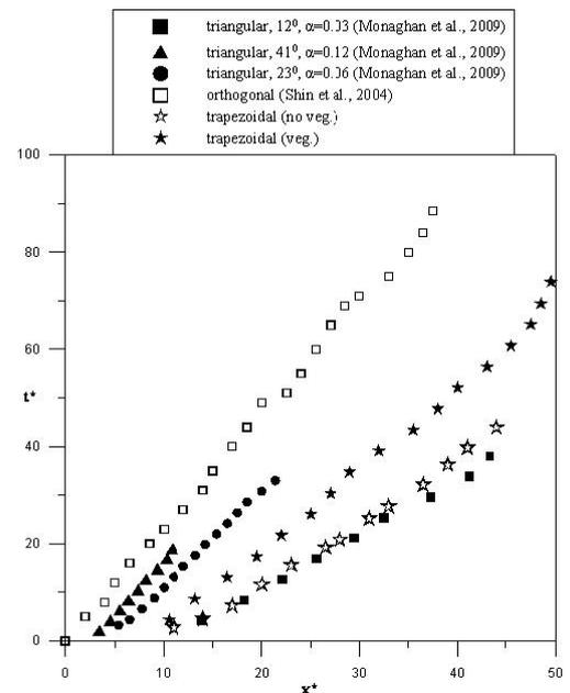
Fig. 4. Time development of gravity front for triangular, orthogonal and trapezoidal cross section (dimensionless).
