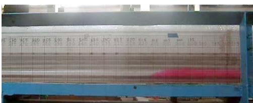
**Photograph 2 Gravity Current (H/H<sub>tr</sub>=1.2 cm, Density Difference 0.3%) at three locations (x=50 cm, x=100 cm, x=170 cm)**
