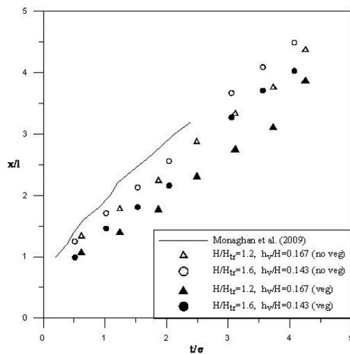
**Fig. 5. Time development of gravity front for a valley of composite cross section (dimensionless).**
