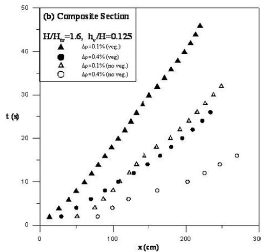
Fig. 2b. Effect of density difference on the motion of gravity current for vegetated and non-vegetated bed for composite section.
