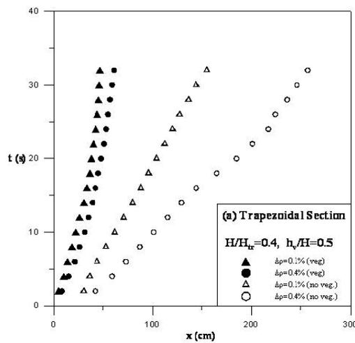
Fig. 2a. Effect of density difference on the motion of gravity current for vegetated and non-vegetated bed for trapezoidal section.
