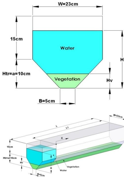
**Fig. 1. Tank dimensions and symbols used.**
