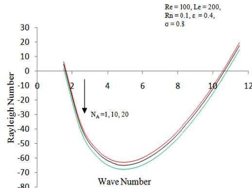
**Fig. 4. Variation of the thermal Rayleigh number ( $Ra_s$ ) with wave number for different value of modified diffusivity ratio.**
