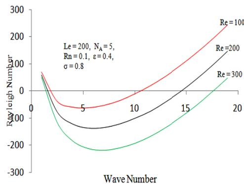
**Fig. 3. Variation of the thermal Rayleigh number ( $Ra_s$ ) with wave number for different value of AC electric Rayleigh number.**
