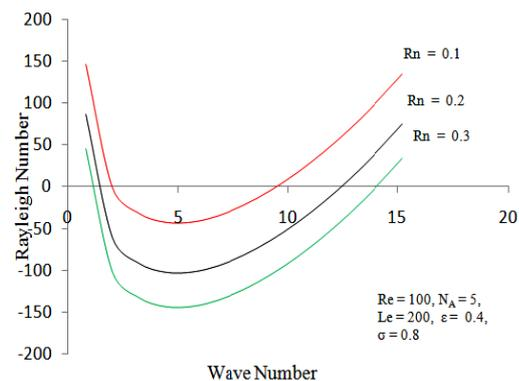
**Fig. 5. Variation of the Rayleigh number ( $Ra_s$ ) with wave number for different value of nanoparticle Rayleigh number.**
