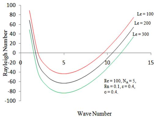
**Fig. 2. Variation of the thermal Rayleigh number ( $Ra_s$ ) with wave number for different value of Lewis number.**
