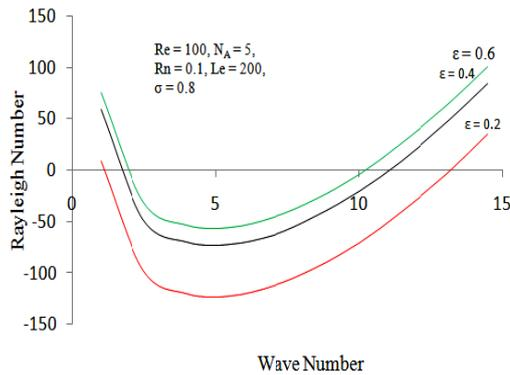
**Fig. 6. Variation of the Rayleigh number (Ra) with wave number for different value of porosity parameter.**
